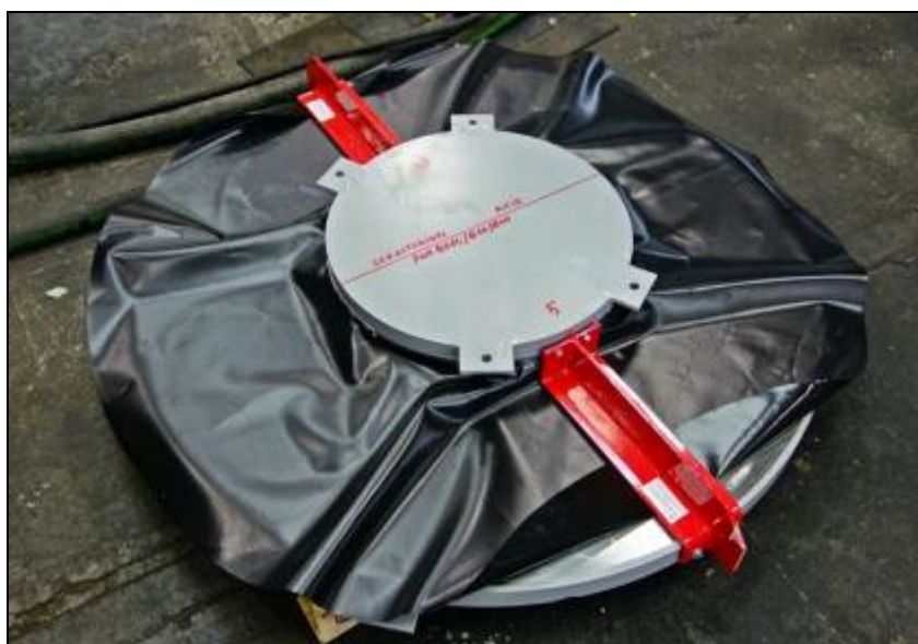
Fig. 13 – Pot bearings installed below walls for stairs and lift
