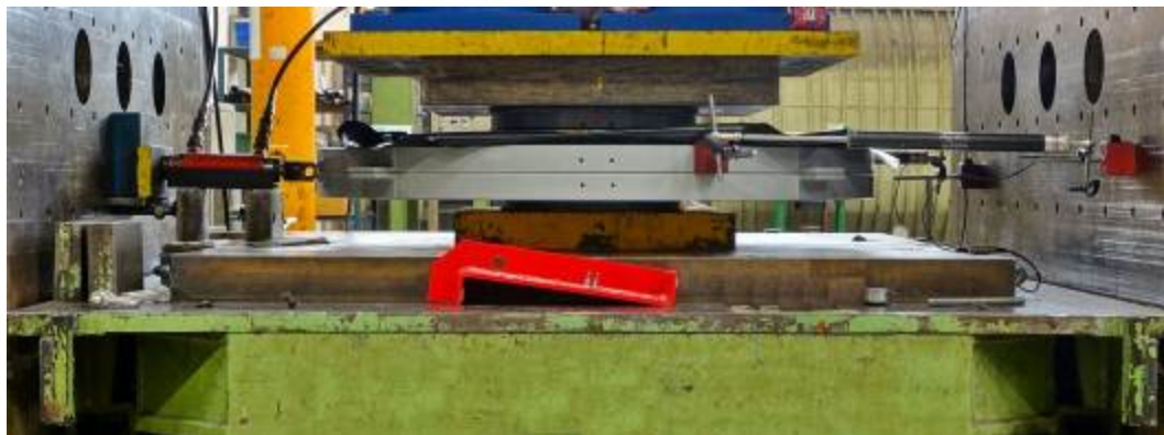
Fig. 16 – Test on Pot bearing at Isolab
