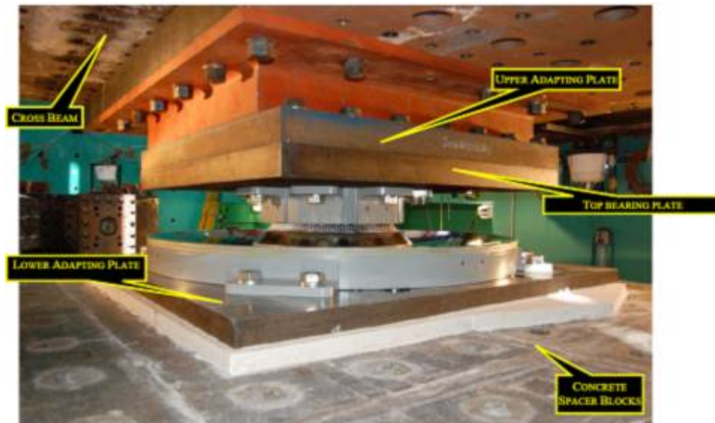
Fig. 12: Test performed on the sliding pendulum at UCSD
