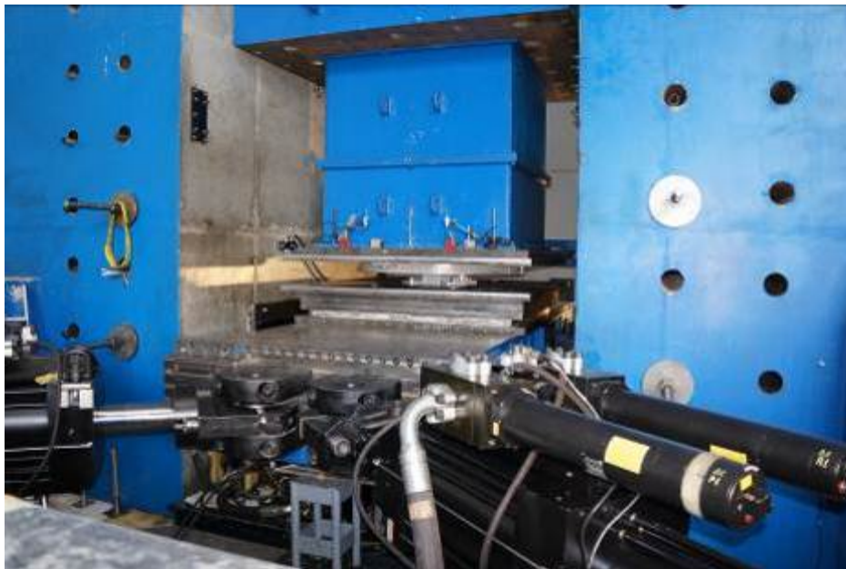
Fig. 13 – Test performed on the sliding pendulum at Eucentre Laboratory
