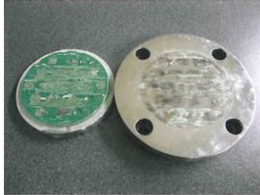
Fig. 9 – Special sliding material “Hotslide” after wear test
