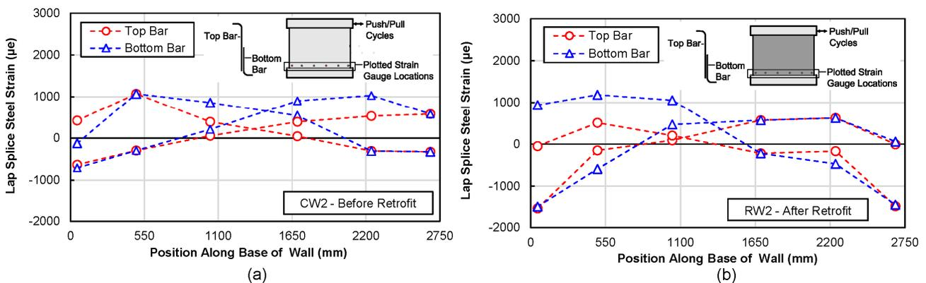
Fig. 9 – Lap splice strain profiles at the maximum load: (a) CW2; (b) RW2
