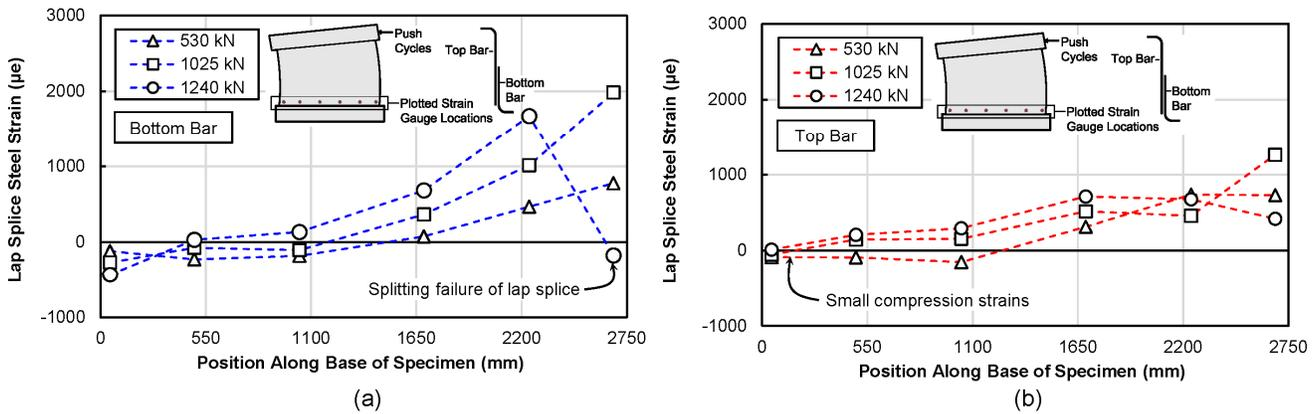
Fig. 7 – Lap splice vertical strain profile for specimen CW3: (a) bottom bar; (b) top bar
