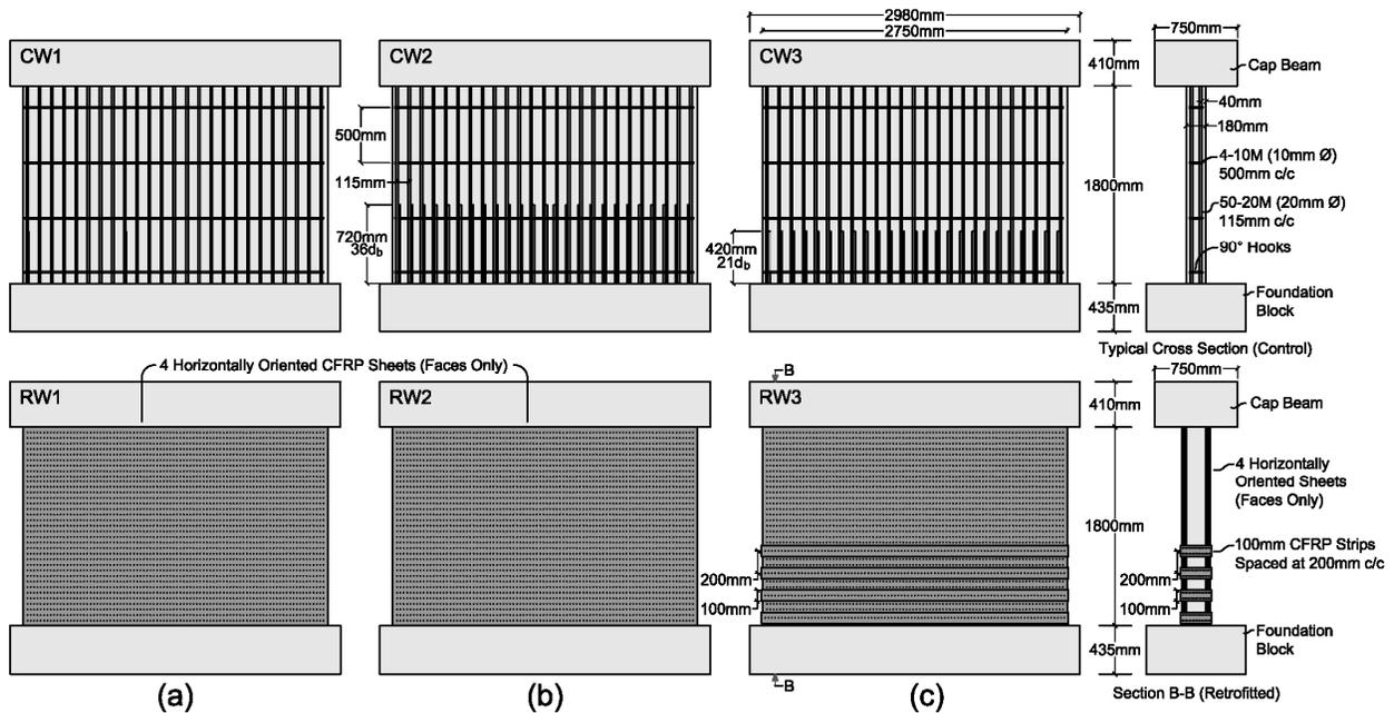
Fig. 3 – Shear wall reinforcement details: (a) CW1/RW1; (b) CW2/RW2; (c) CW3/RW3
