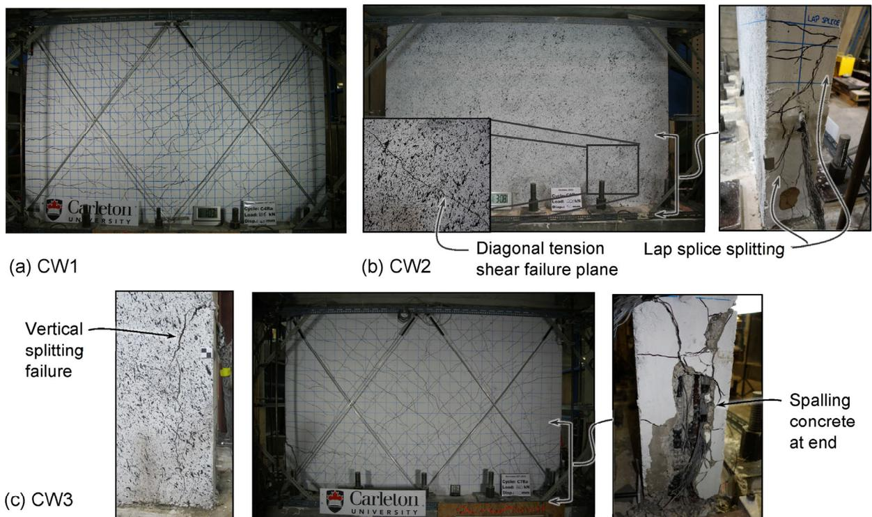
Fig. 6 – Damage to control specimens: (a) CW1; (b) CW2; (c) CW3
