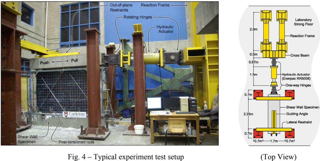
Fig. 4 – Typical experiment test setup
