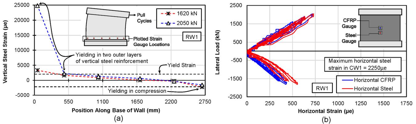
Fig. 8 – Strain distributions in specimen RW1: (a) vertical strain profiles; (b) horizontal strain hysteresis
