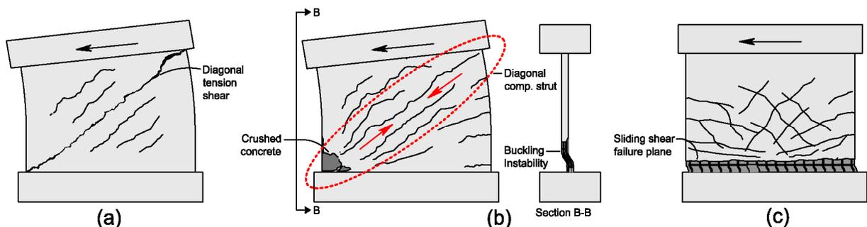
Fig. 1 – Shear wall failure modes: (a) diagonal tension; (b) diagonal compression; (c) sliding shear
