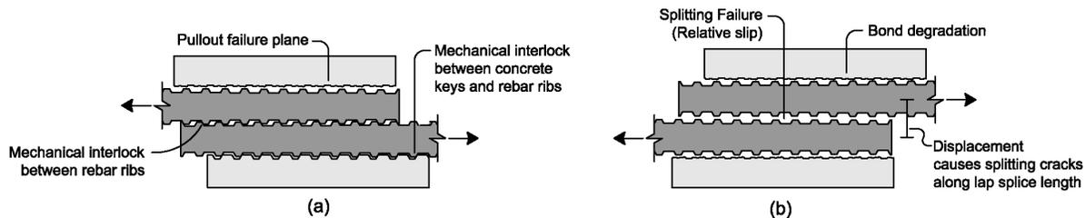
Fig. 2 – Lap splice failure mechanisms: (a) pullout failure; (b) splitting failure
