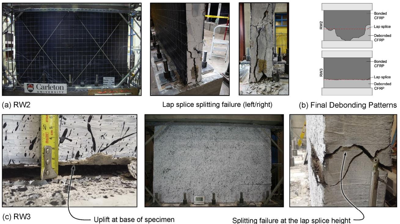
Fig. 10 – Damage to retrofitted wall specimens with lap splices: (a) RW2; (b) debonding pattern; (c) RW3
