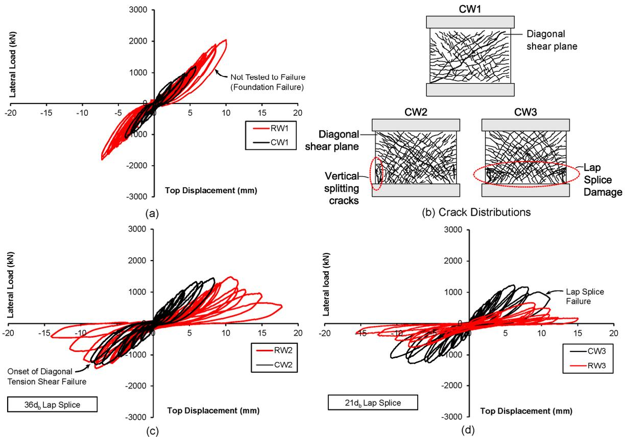
Fig. 5 – Hysteretic response behavior: (a) CW1/RW1; (b) crack distributions; (c) CW2/RW2; (d) CW3/RW3
