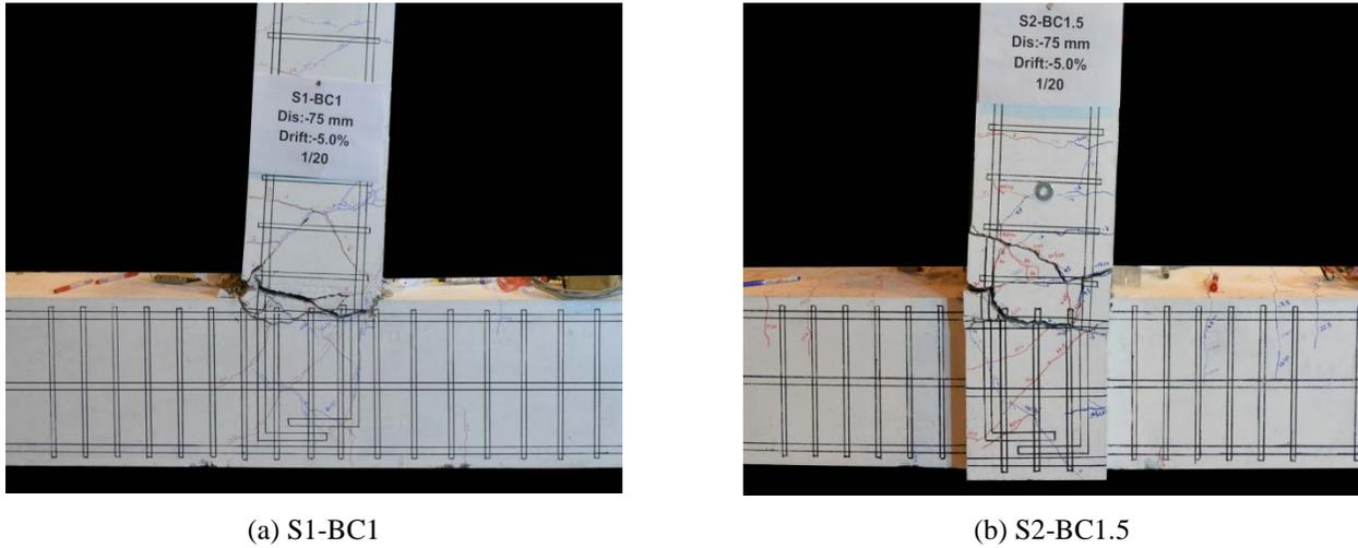
Fig. 7 – Crack patterns of tested specimens at 5% drift ratio
