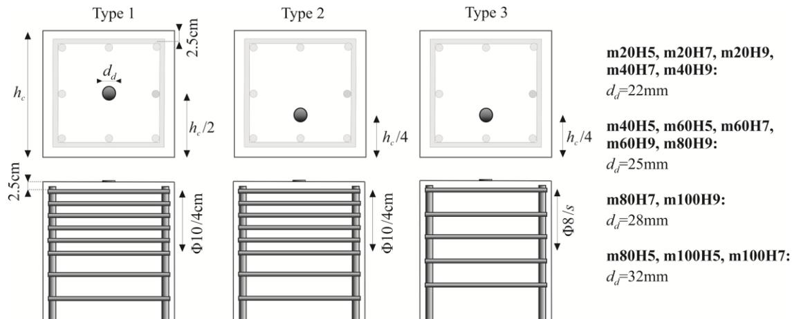
Fig. 3 – The three different types of the analyzed dowel connections.
