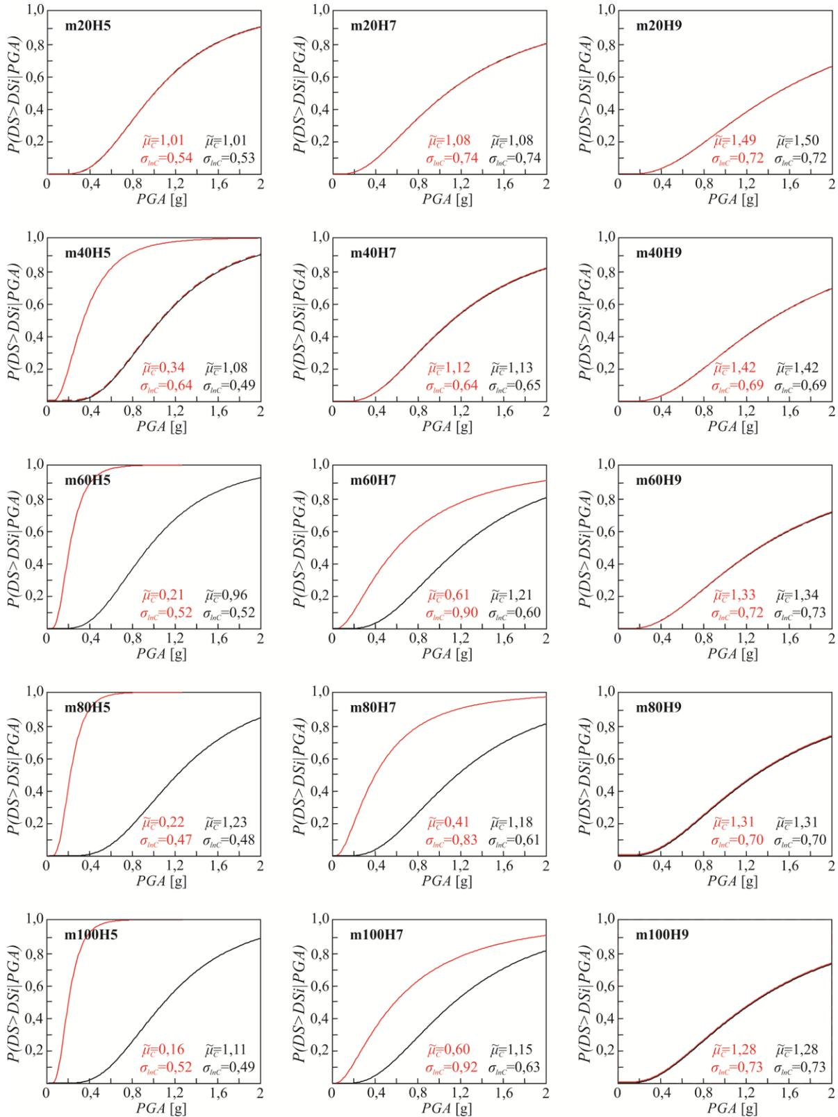
Fig. 7 – Fragility curves for buildings with “strong” (black curves) and “weak” (red curves) centric dowel connections – type 1 (see Fig. 3). It is assumed that only one beam is connected to a column.
