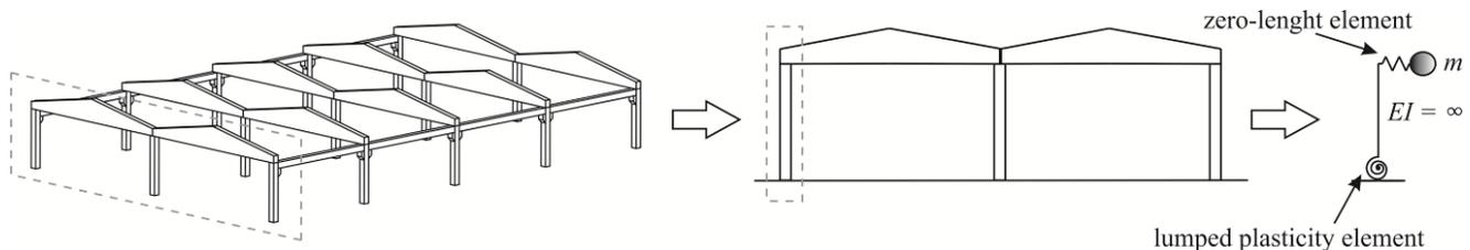
Fig. 4 – Nonlinear model of the single-storey industrial building taking into the account nonlinear response of columns and beam-column dowel connections.
