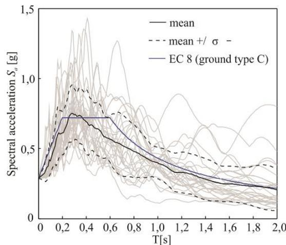
Fig. 6 – Spectra of the selected 30 ground-motion records and the Eurocode 8 spectrum for soil type C.
