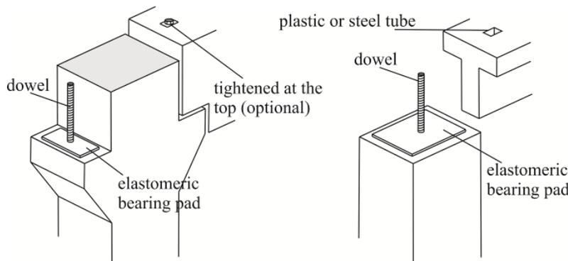
Fig. 1 – The scheme of the beam-column dowel connection assembly.
