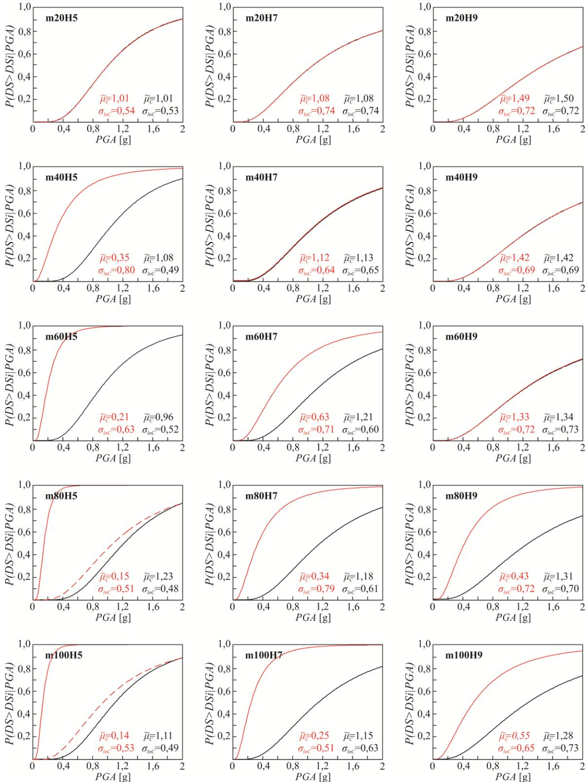
Fig. 8 – Fragility curves for buildings with “strong” (black curves) and “weak” (red curves) eccentric dowel connections with a relatively large amount of stirrups around the dowel – type 2 (see Fig. 3). It is assumed that one (continuous red curves) or two beams (dashed red curves) are connected to a column.
