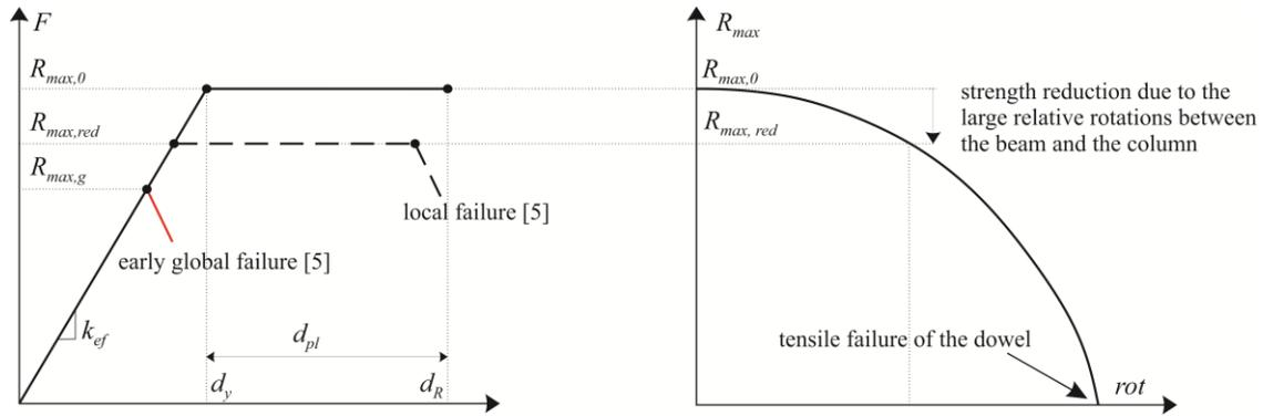
Fig. 5 –Force-displacement response envelope of dowel connections (left) and strength reduction due to the large relative rotations between the beam and the column (right)
