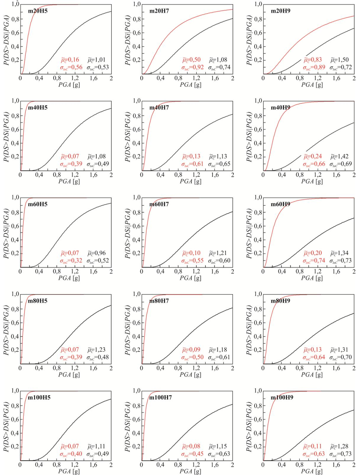
Fig. 9 – Fragility curves for buildings with “strong” (black curves) and “weak” (red curves) eccentric dowel connections with a relatively small amount of stirrups around the dowel – type 3 (see Fig. 3). It is assumed that only one beam is connected to a column.
