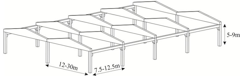
Fig. 2 – Structural system of the analyzed single-story precast industrial buildings.
