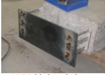
(a) Welded steel plate
