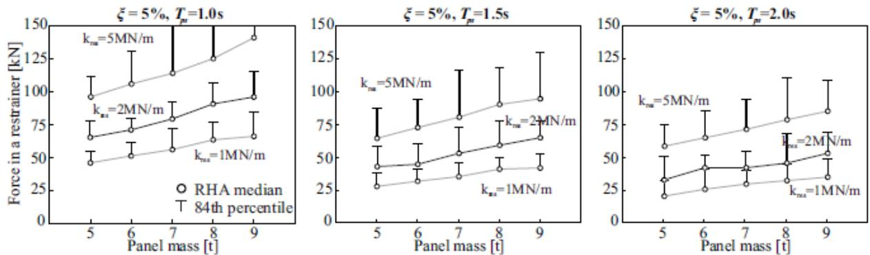
Fig. 13 Results of the RHA: the maximum impact forces in a restrainer for different input parameters, including the panel mass, the restrainer stiffness  $k_{res}$ , period of the primary structure  $T_{ps}$  and an assumed damping ratio of  $\xi = 5\%$ .
