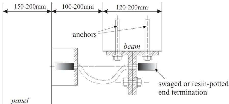
Fig. 3 A scheme of a restrainer system as a second-line back-up device for the prevention of the collapse of concrete cladding panels in the case of seismic events
