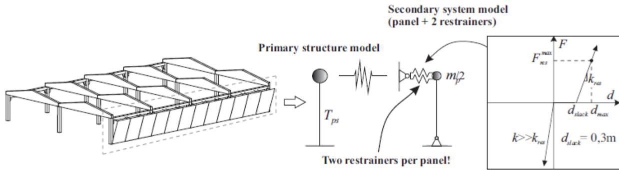
Fig. 9 Models of the primary structure and of the secondary system (panel and 2 restrainers)
