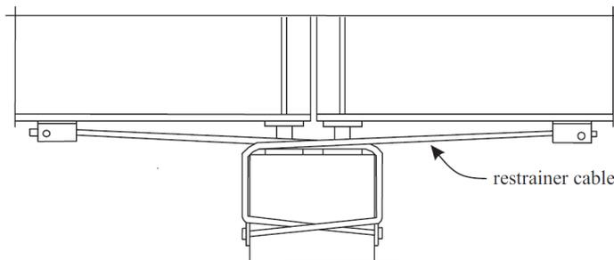
Fig. 1 A scheme of a restrainer system that is typically used for the seismic protection of multi-span simply supported bridges [6]
