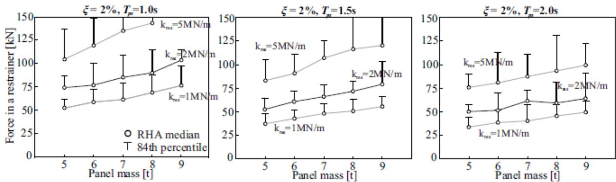
Fig. 12 Results of the RHA: the maximum impact forces in a restrainer for different input parameters, including the panel mass, the restrainer stiffness  $k_{res}$ , period of the primary structure  $T_{ps}$  and an assumed damping ratio of  $\xi = 2\%$ .
