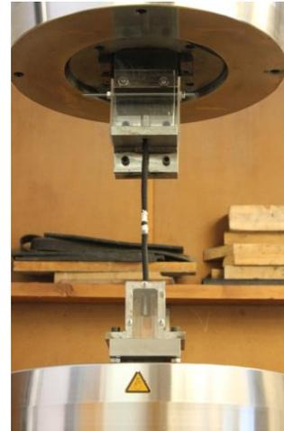
Fig. 5 The test of the capacity and stiffness
