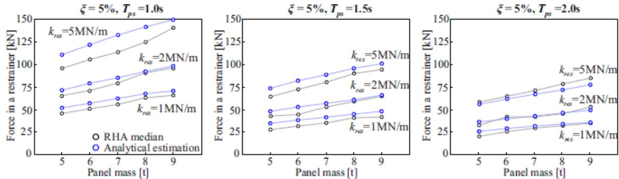
Fig. 16 The match between the numerically obtained maximum forces in restrainers and maximum forces in restrainers derived using the proposed analytical formula
