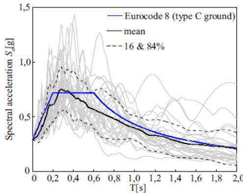
Fig. 10 Spectra for the set of 30 selected accelerograms and the target Eurocode 8 spectrum
