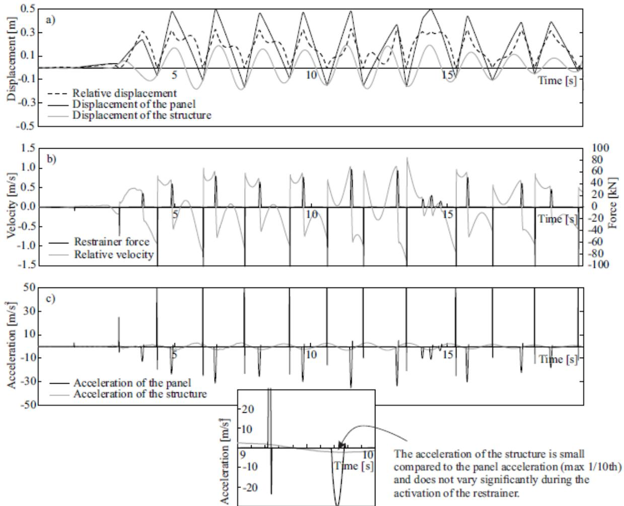
Fig. 11 Results of RHA for a single accelerogram: response history for displacements, accelerations, relative velocity, and the impact force acting in the restrainer
