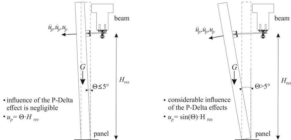
Fig. 7 The response of short (left) and long restrainers (right): Short restrainers do not permit any larger inclination of the panel - the P-Delta effect is therefore small or negligible. (left) Long restrainers permit significant inclination of the panel, so the P-Delta effect should be taken into account when estimating the maximum impact forces in the restrainers (right)
