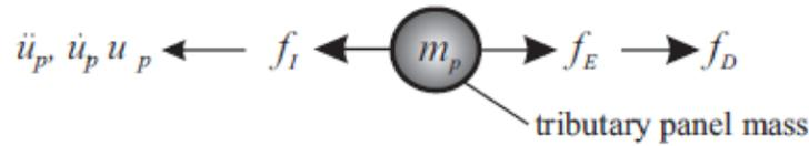
Fig. 8 An analytical model which can be used to estimate the maximum impact forces in restrainers ( $u_p$ ,  $\dot{u}_p$  and  $\ddot{u}_p$  are the displacement, velocity, and acceleration of the panel at the height of the restrainer;  $f_I$ ,  $f_E$  and  $f_D$  are the inertial, internal, and damping forces).
