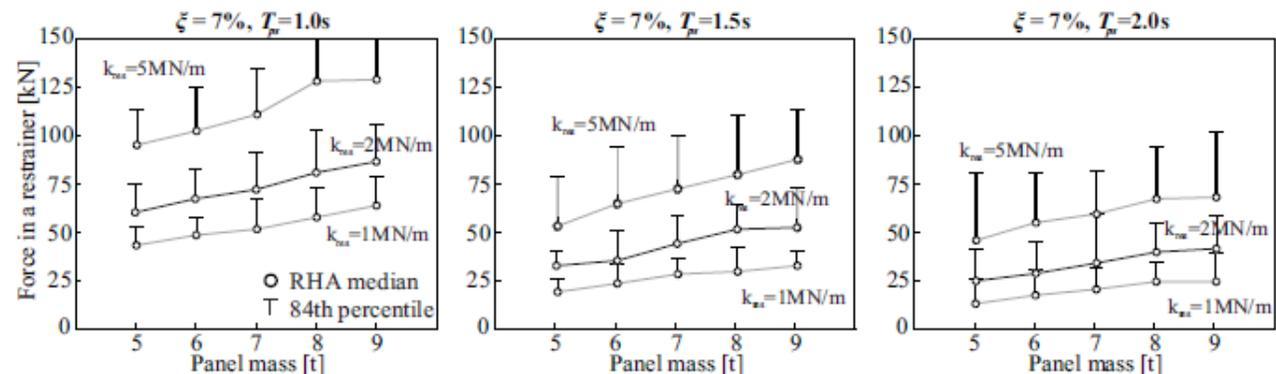
Fig. 14 Results of the RHA: the maximum impact forces in a restrainer for different input parameters, including the panel mass, the restrainer stiffness  $k_{res}$ , period of the primary structure  $T_{ps}$  and an assumed damping ratio of  $\xi = 7\%$ .
