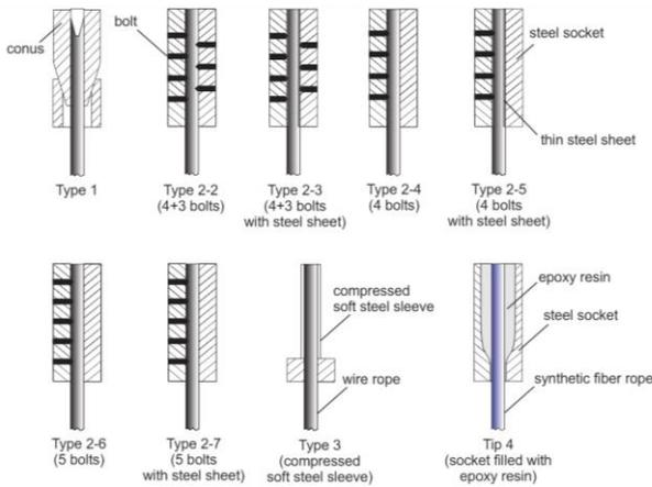
Fig. 4 Different terminations of the examined ropes
