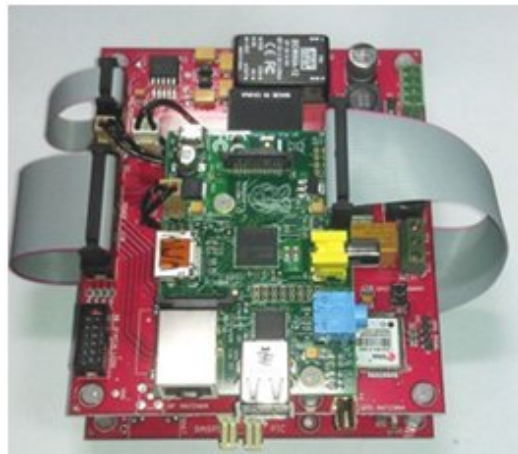
Fig 1 – Internal view of DAC type strong motion accelerometer
