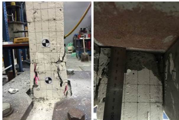
Fig. 9 Damage of column 7seg (column base; column top)
