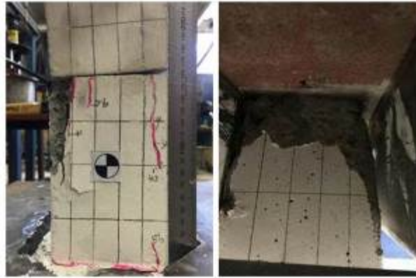
Fig. 6 Damage of column 5seg (column base and column top)
