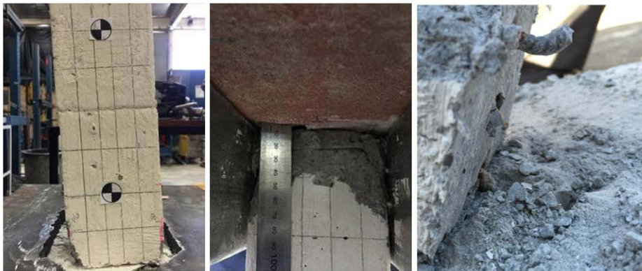
Fig. 7 Damage of column 5segED (column base; column top; fracture of starter bar)
