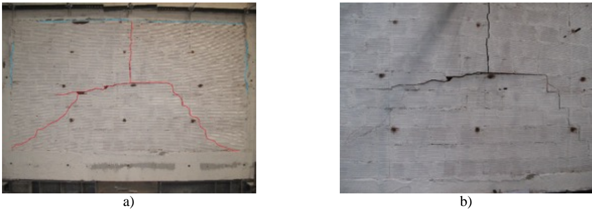
Fig. 9 – Inf_02: a) Cracking pattern; and b) Trilinear cracking pattern observed in the center of the panel.
