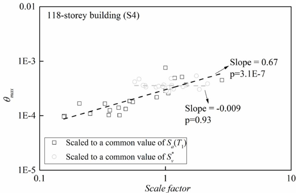
Fig. 6 –  $\theta_{max}$  versus record scale factor
