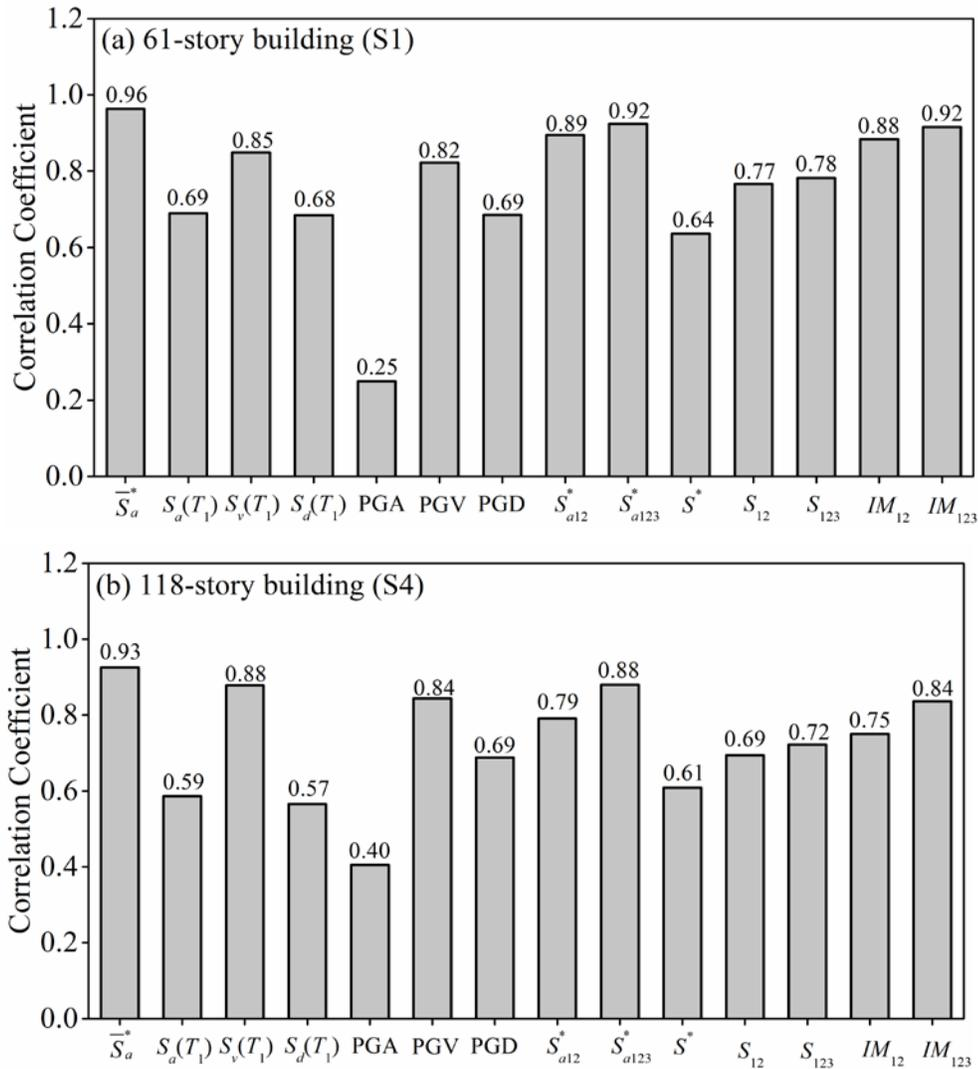
Fig. 5 – The correlation between  $\theta_{max}$  and IMs under given M, R for sufficiency
