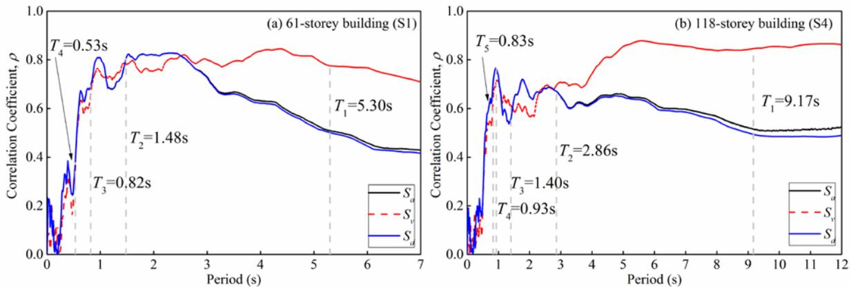
Fig. 2 – The correlation of  $S_a$ ,  $S_v$  and  $S_d$  to  $\theta_{\max}$  of the two buildings
