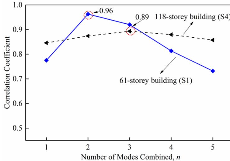
Fig.3 – Correlation coefficients between  $\theta_{max}$  and  $S_v^*$  with different combinatorial terms
