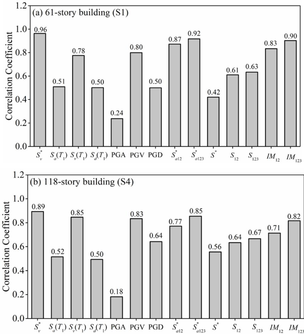
Fig. 4 – The correlation between  $\theta_{max}$  and IMs for efficiency
