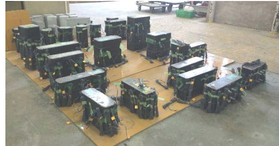
Fig. 3 – Specimens with strain gauges
