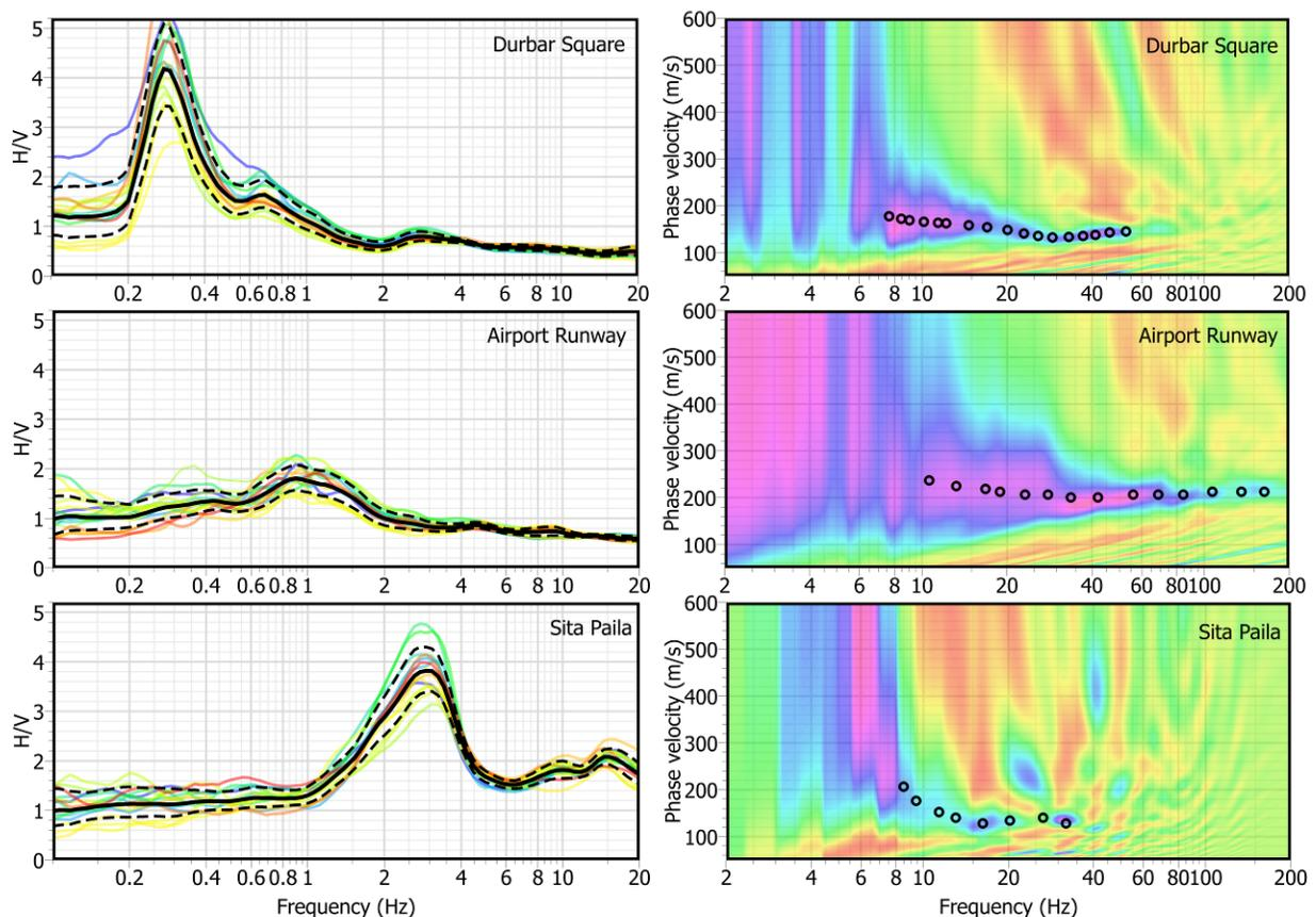
Figure 6. Average microtremor HVSRs (left) and dispersion curves (right) at three select locations in the Kathmandu Valley.
