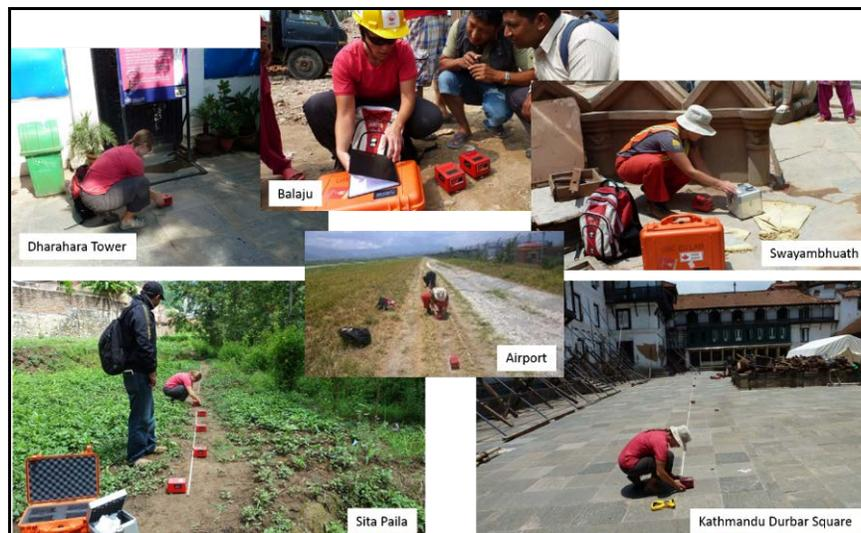
Figure 2. Photos of microtremor measurements performed in and around Kathmandu using ultra-portable TROMINO<sup>®</sup> sensors.
