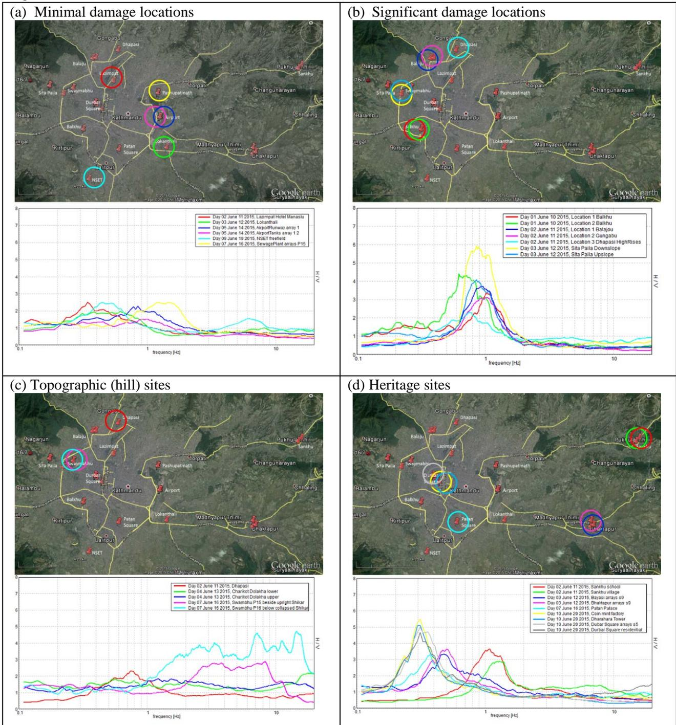
Figure 3. Microtremor HVSR response (amplification vs. frequency) measured in locations (a) of minimal and (b) significant observed damage in Kathmandu, as well as (c) at topographic hill and (d) heritage sites around Kathmandu. Colour corresponds to circled locations shown in maps above each plot.
