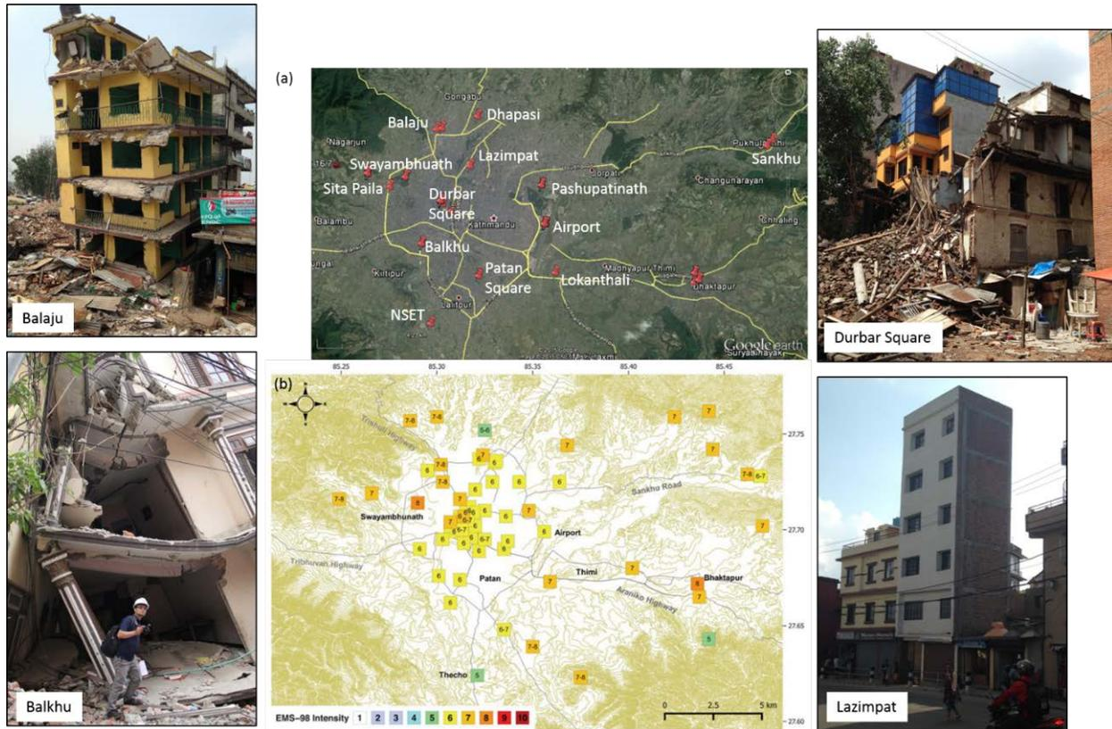
Figure 1. (a) Sites visited in and around central Kathmandu by the CAEE reconnaissance team marked by red pushpins. (b) Macroseismic EMS-98 intensity map of the M 7.8 Gorkha earthquake [8]; Fig. 2.
