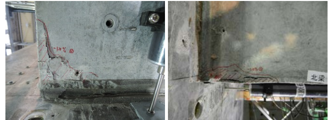
(a) Bottom face of beam (b) Side face of (a) Photo 1 Compressive damage of concrete ( R=1.0\% )
