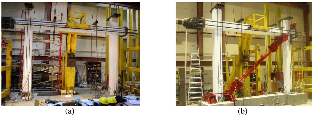
Fig. 3 - Setup prior to testing: a) control frame; and b) retrofitted frame
