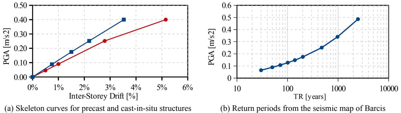
Fig. 6 – Relations between PGA and IDR (a) and between PGA and return period (b)
