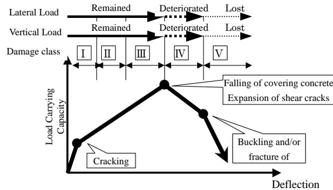
Fig. 7–Idealized lateral force-displacement relationships and damage class[2]
