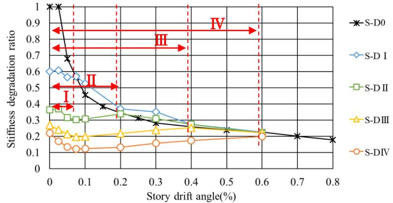
Fig.12–Stiffness degrading ratio
