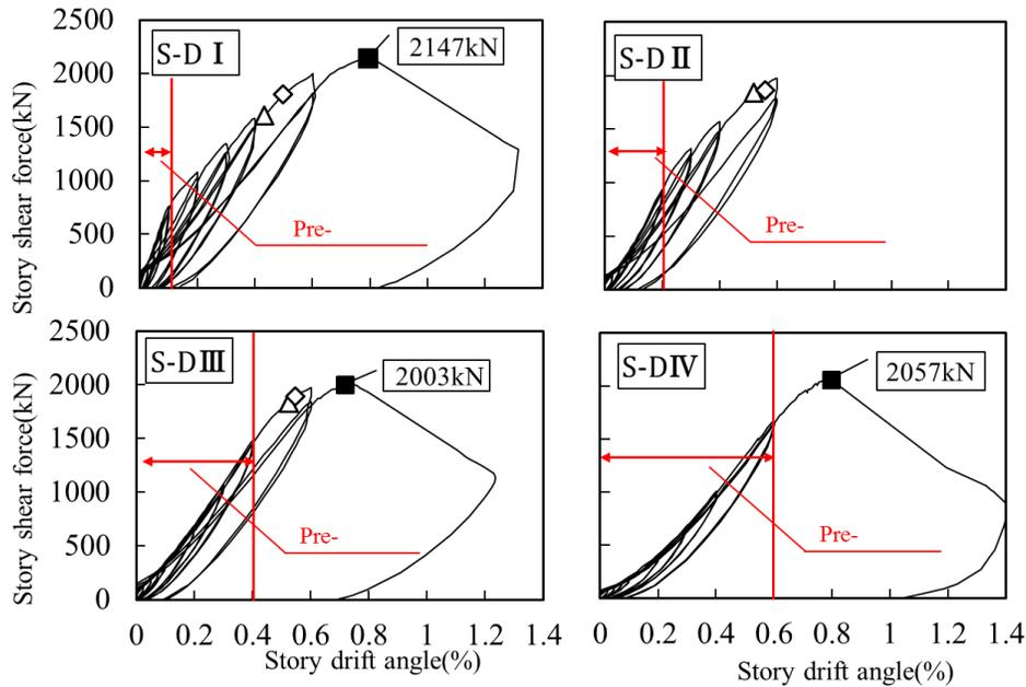
Fig.10–Shear force-story drift angle relationship of damaged specimens
