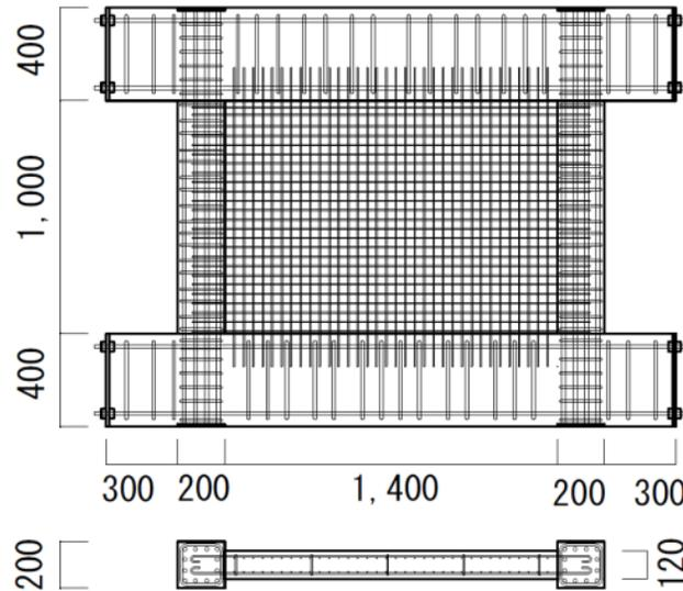
Fig. 1 – Reinforcing detail of specimen: elevation and section
