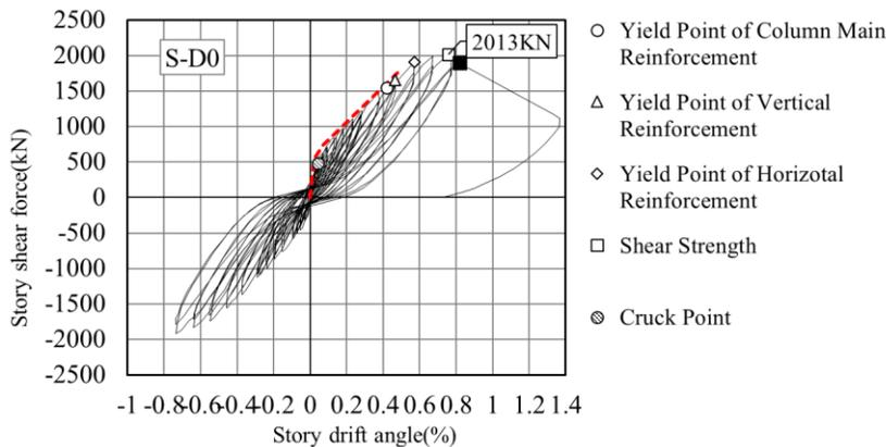
Fig. 4– Shear force-story drift angle relationship of S-D0
