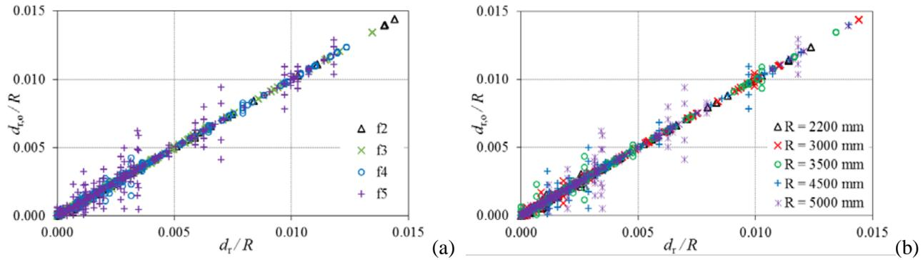
Fig. 5 – Influence of the initial offset on the residual displacement: dependence on the friction (a), on the radius of curvature of the CSS isolator (b)
