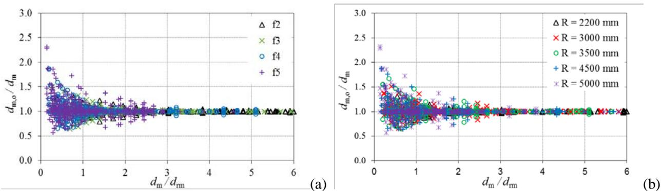
Fig. 4 – Influence of the initial offset on the maximum displacement: dependence on the friction (a), on the radius of curvature of the CSS isolator (b)
