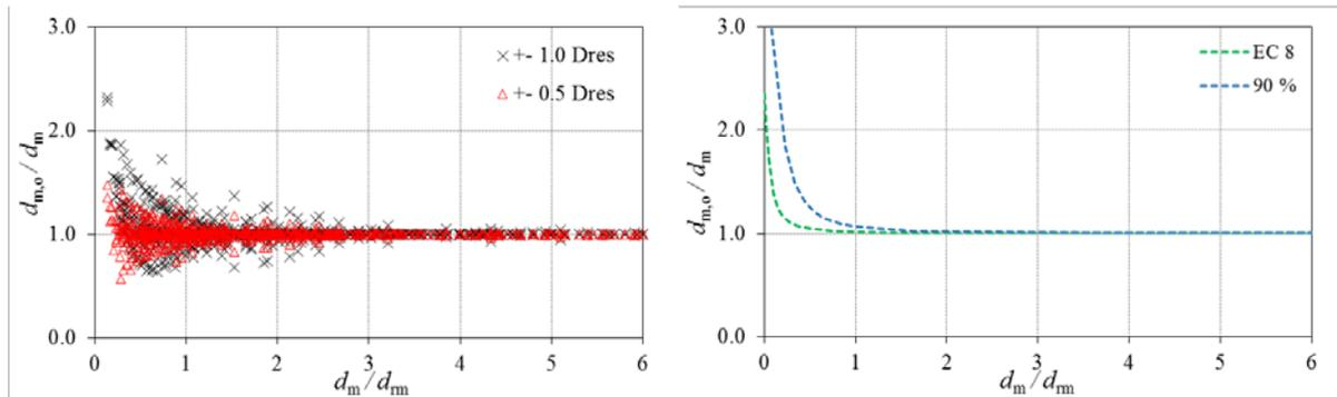
Fig. 3 – Influence of the initial offset on the maximum displacement increase (left) and comparison (at 90% percentile) with EC 8 (right)
