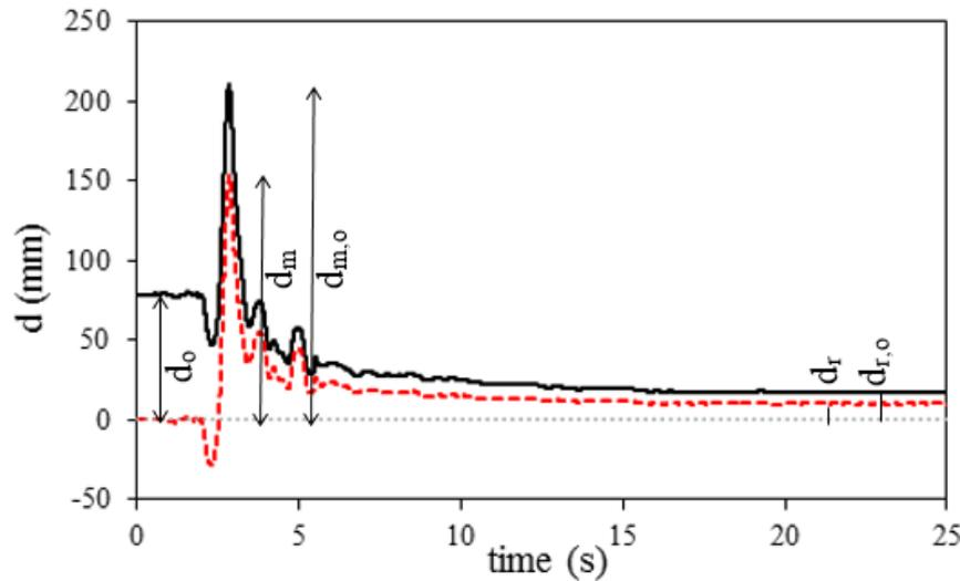
Fig. 2 – Time-histories displacement response parameters of the isolated structure with initial offset (solid black line) and without initial offset (dotted red line)
