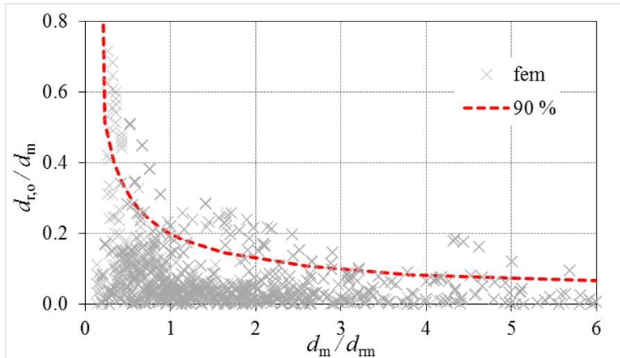
Fig. 6 – Influence of the initial offset on the re-centring capability and the 90<sup>th</sup> percentile of non linear response analysis results
