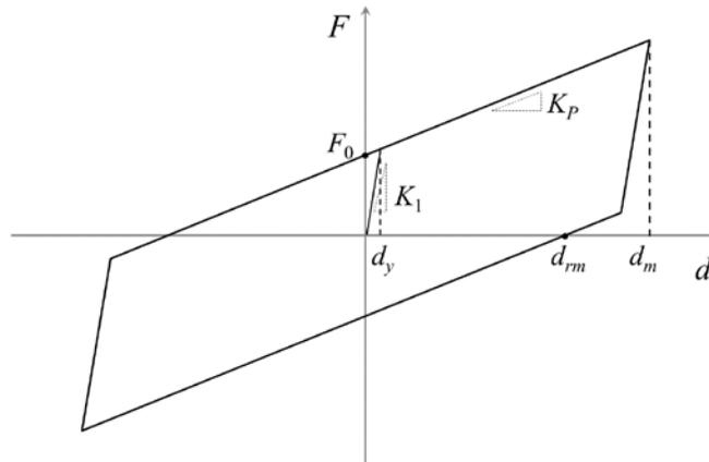
Fig. 1 – Force – displacement characteristic of a bilinear hysteretic isolation system
