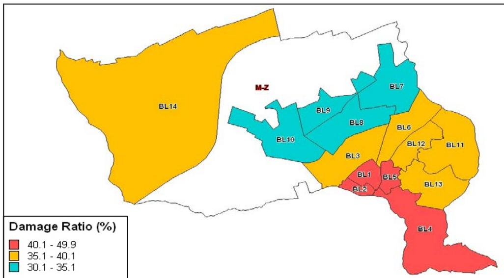
Fig. 13 – Mean damage ratio in each sector of Blida city
