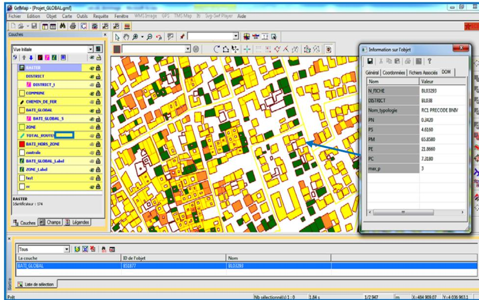
Fig. 9 – Generation of a GIS damage map (classification of the building according to the preponderant damage level)
