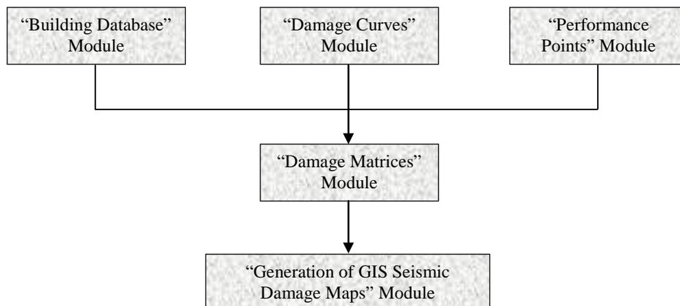
Fig. 3 – Flow chart of the Rapid earthquake loss estimation model for building in Algeria
