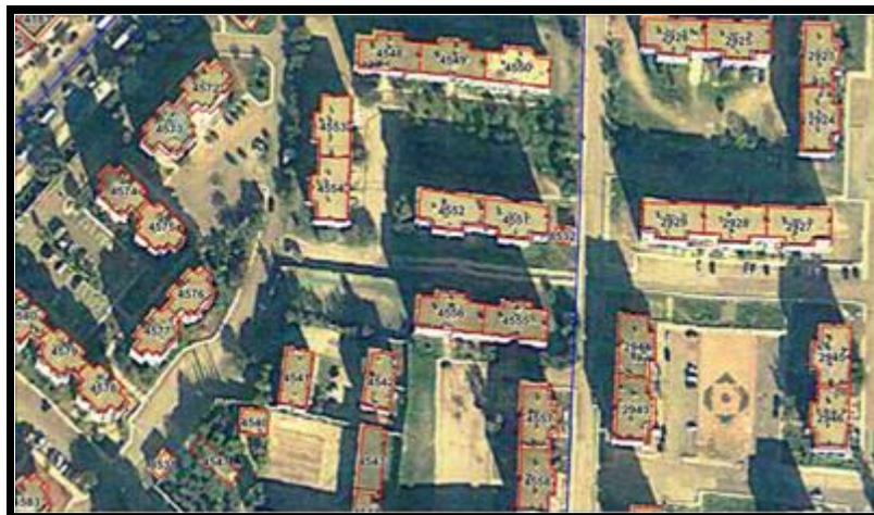
Fig. 11 – Example of the digitised buildings of Blida city in GIS platform using high-resolution Geo-Eye satellite imagery
