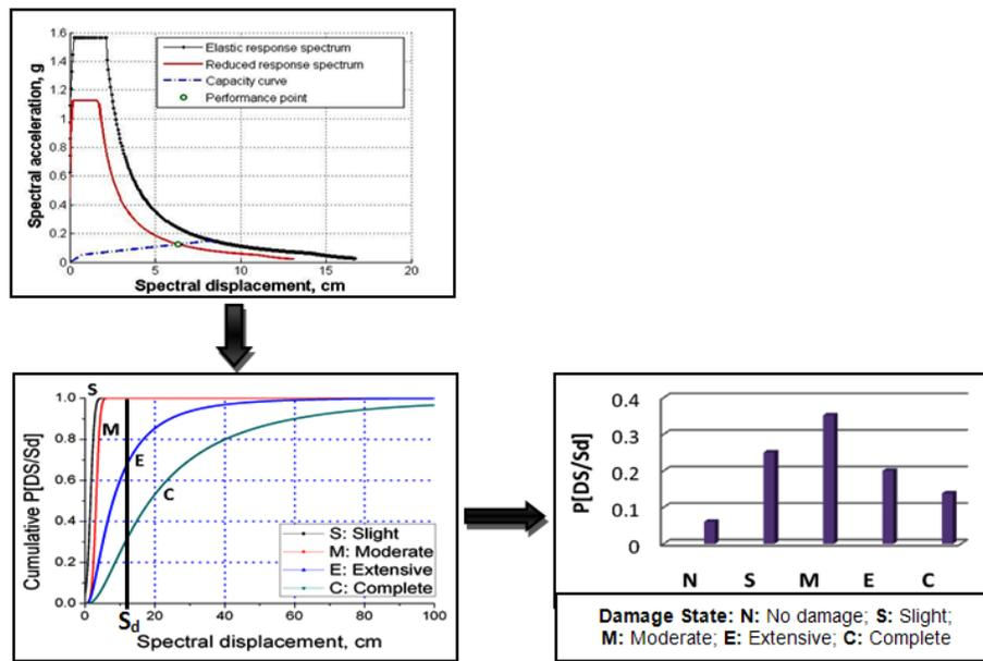
Fig. 2 – Schematization of the seismic damage estimation process of existing buildings in Algeria [1, 2]
