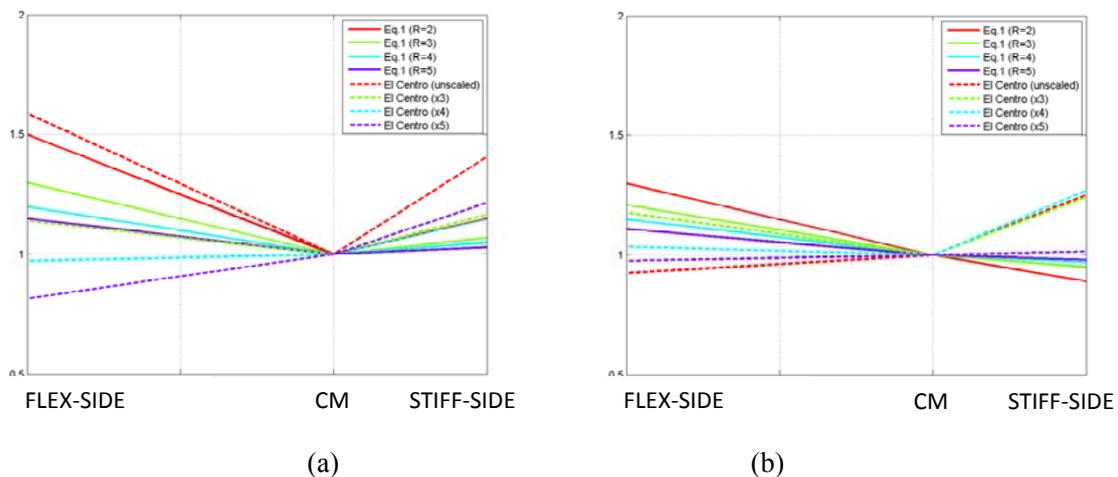
Fig. 13 – Normalized displacements  $u_{\max}/u_{CM,\max}$  in the horizontal plane at the top of buildings and predictions according to Eq. (1): (a) F-15 building; (b) S-15 building.
