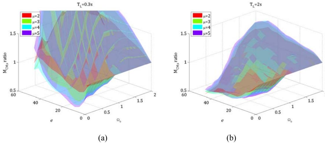
Fig. 7 – Surfaces of  $M_{CM,s}$  ratio: nonlinear systems / linear response. (a)  $T_L=0.3$  s and (b)  $T_L=2$  s.
