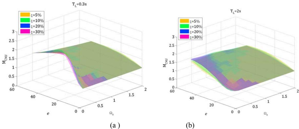
Fig. 2 – Surfaces of  $M_{CM,f}$  for linear systems with (a)  $T_L=0.3$  s and (b)  $T_L=2$  s.
