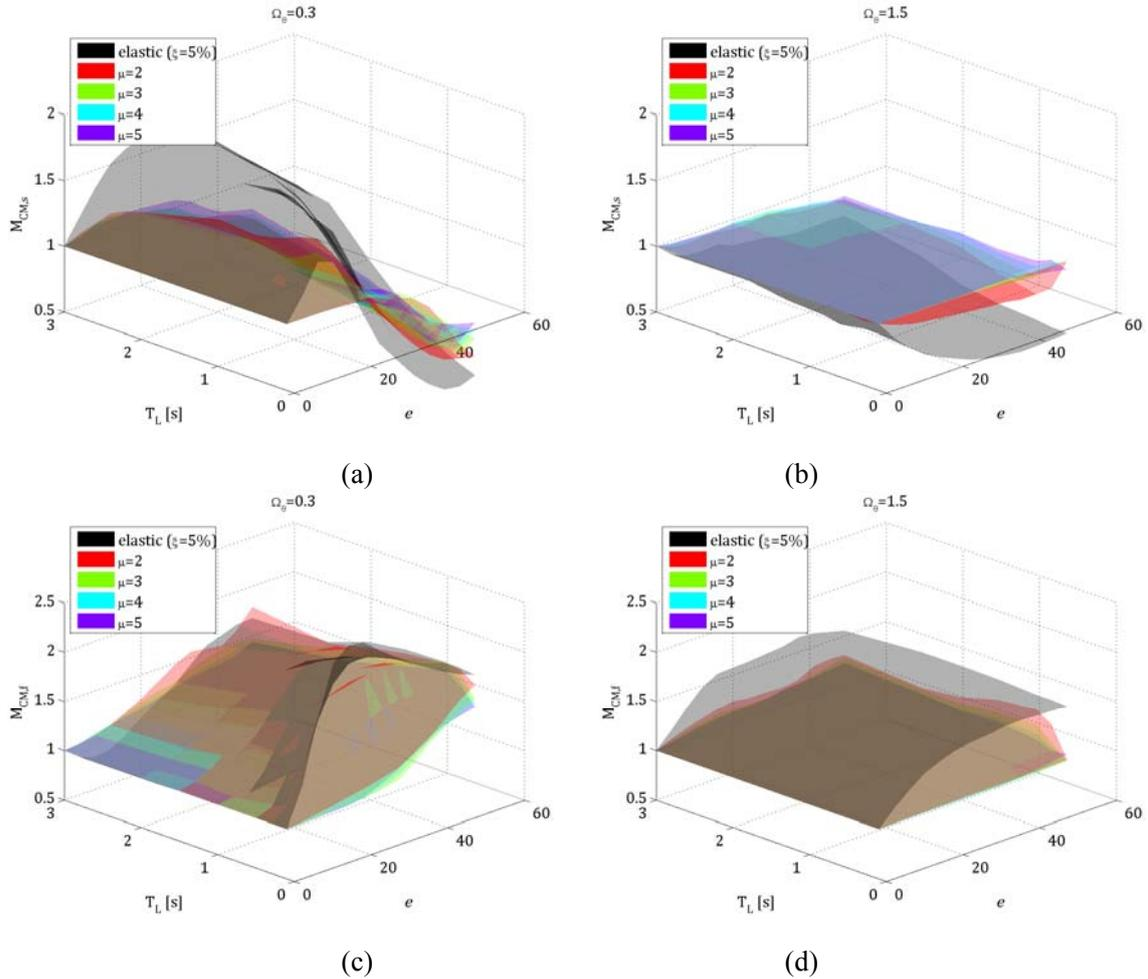
Fig. 8 – 3D spectra of: (a)  $M_{CM,s}$  for torsionally flexible system with  $\Omega_\theta=0.3$ ; (b)  $M_{CM,s}$  for torsionally stiff system with  $\Omega_\theta=1.5$ ; (c)  $M_{CM,f}$  for torsionally flexible system with  $\Omega_\theta=0.3$ ; (d)  $M_{CM,f}$  for torsionally stiff system with  $\Omega_\theta=1.5$ .
