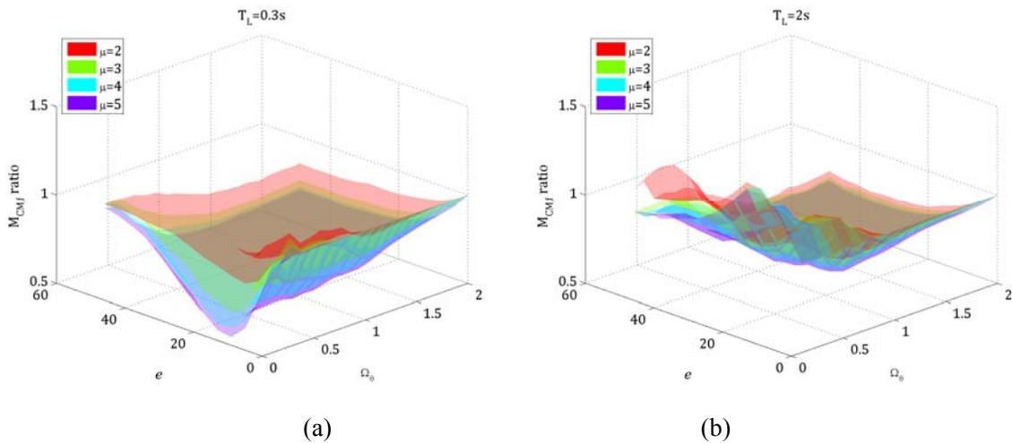
Fig. 6 – Surfaces of  $M_{CM,f}$  ratio: nonlinear systems / linear response. (a)  $T_L=0.3$  s and (b)  $T_L=2$  s.
