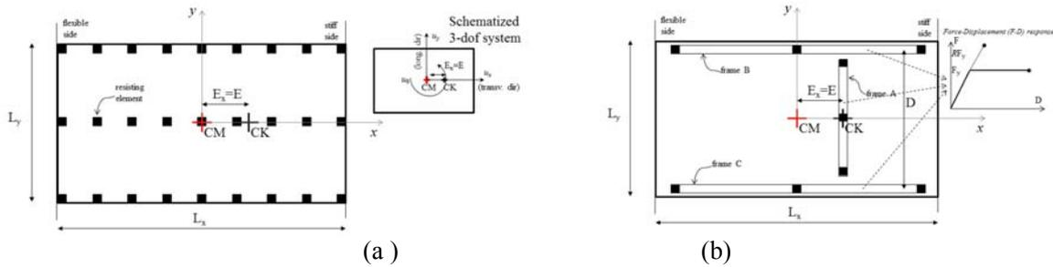
Fig. 1 – Linear (a) and non-linear (b) one-storey asymmetric system.
