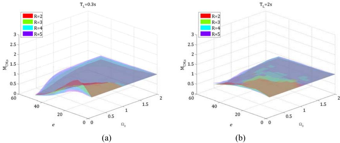
Fig. 5 – Surfaces of  $M_{CM,s}$  for nonlinear systems with (a)  $T_L=0.3$  s and (b)  $T_L=2$  s.
