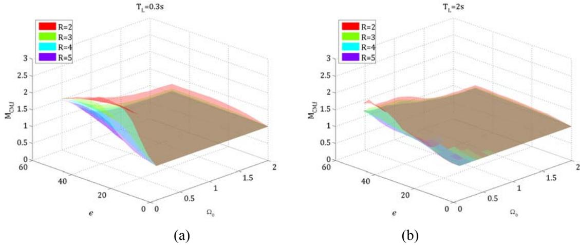
Fig. 4 – Surfaces of  $M_{CM,f}$  for nonlinear systems with (a)  $T_L=0.3$  s and (b)  $T_L=2$  s.
