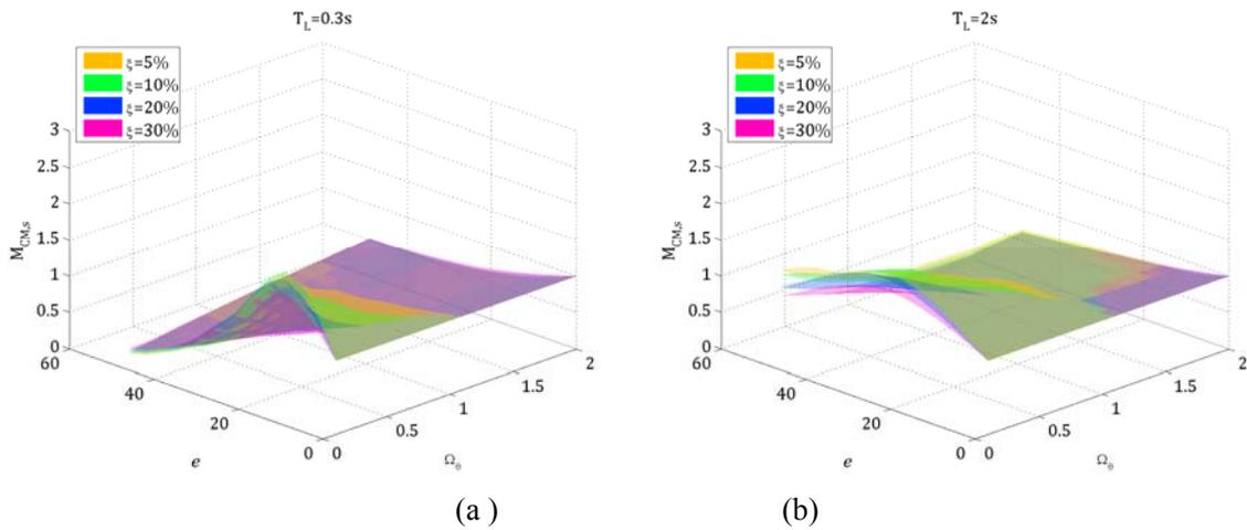
Fig. 3 – Surfaces of  $M_{CM,s}$  for linear systems with (a)  $T_L=0.3$  s and (b)  $T_L=2$  s.
