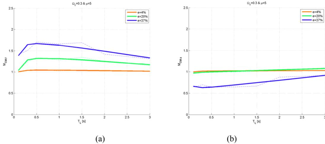
Fig. 10 – (a)  $M_{CM,f}$  and (b)  $M_{CM,s}$  according to Eq. (3) compared with the corresponding numerical spectra.
