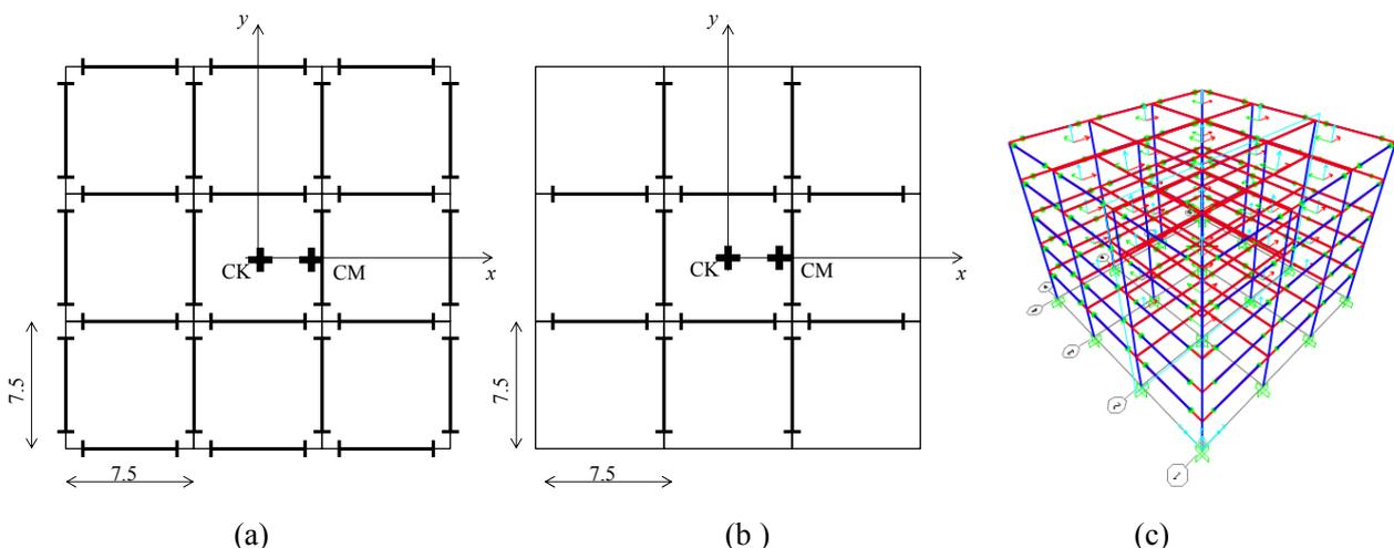
Fig. 12 – Schematic plans of (a) S-15 and (b) F2-15. (c) SAP 2000 model of F2-15.
