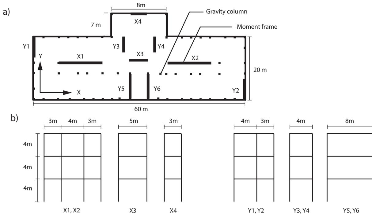
**Fig 1** – Case study office building a) typical plan b) elevation of moment frames
