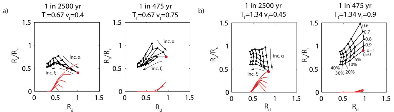
**Fig 3 – Viscous-viscoelastic P-Spectra for a) stiff frame and b) flexible frame**
