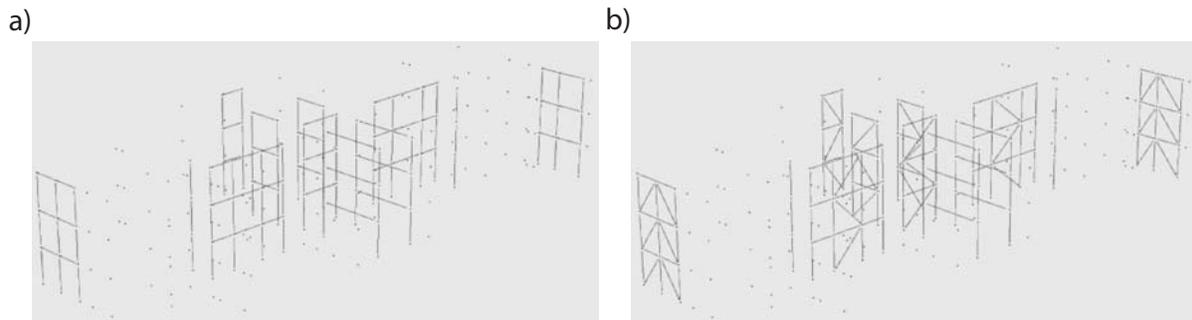
**Fig 5** – Perform3D model of 3 storey office a) base frame b) with supplemental dampers
