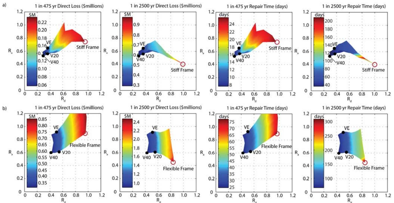
**Fig 4** – P-Spectra direct loss and downtime contour for a) stiff frame and b) flexible frame
