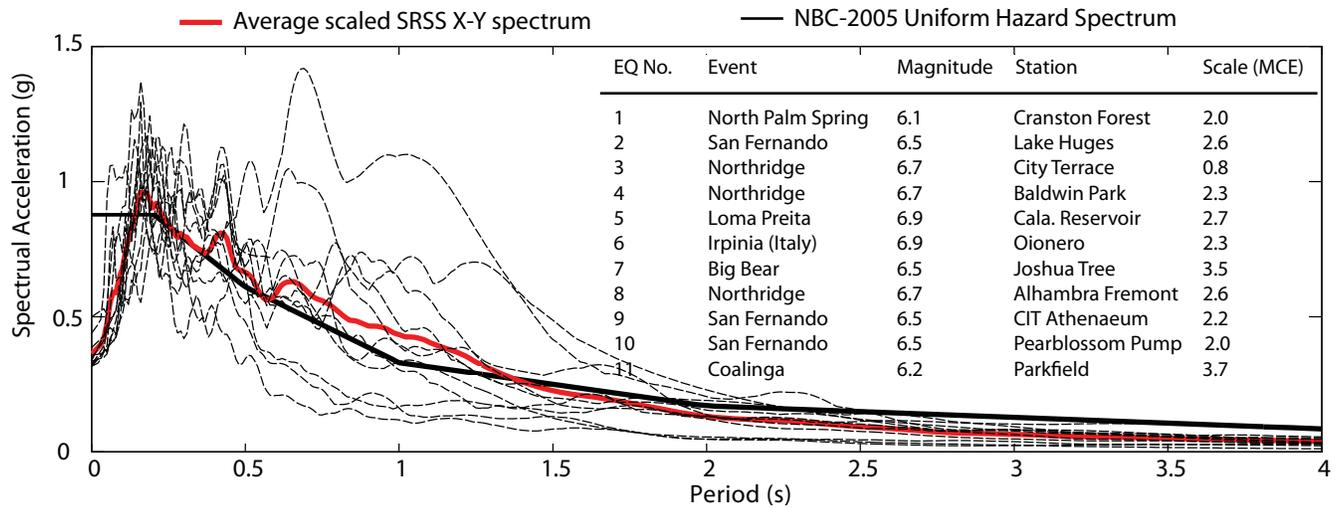
Fig 2 – Design NBCC2005 UHS and scaled suite of 11 pairs of ground motion
