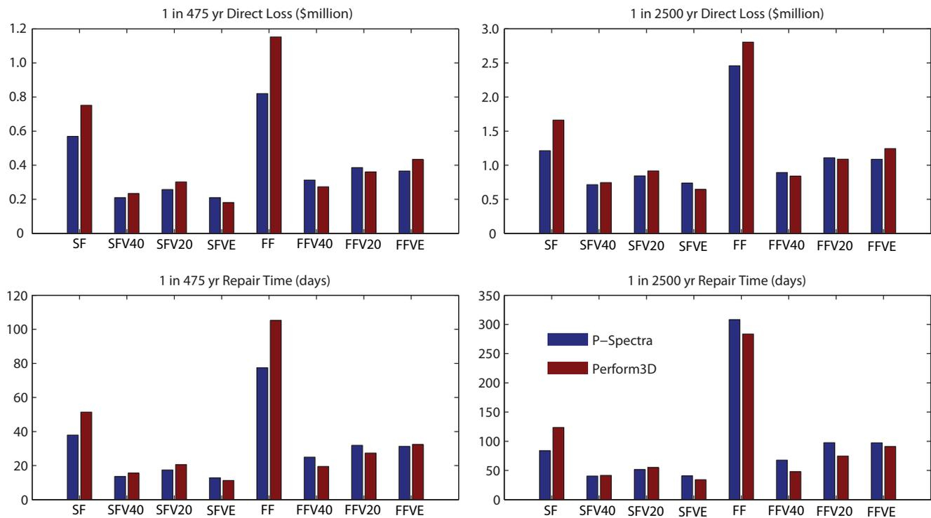
**Fig 6** – Comparison of direct losses and downtime computed from P-Spectra and nonlinear time-history
