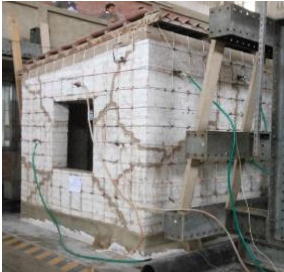
Figure 3 – Full-scale adobe model reinforced with nylon-rope mesh (credits: Blondet et al. 2013)
