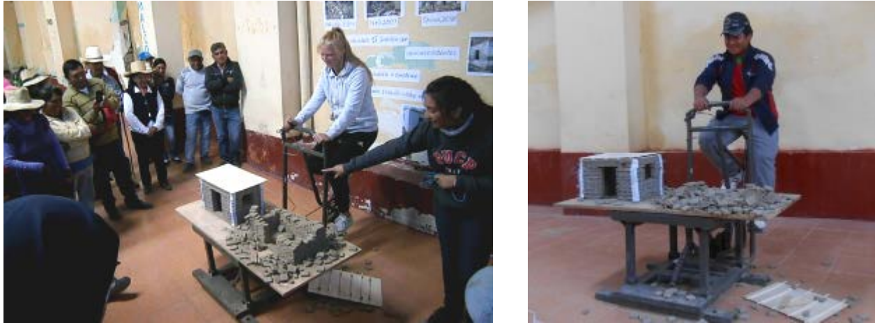
Figure 10 – Live portable shaking table demonstrations
