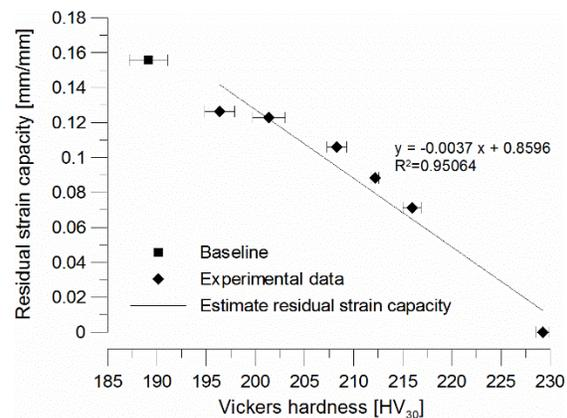
Fig. 10 Residual strain capacity versus Vickers hardness calibration curve for diameter 16 mm grade 430.
