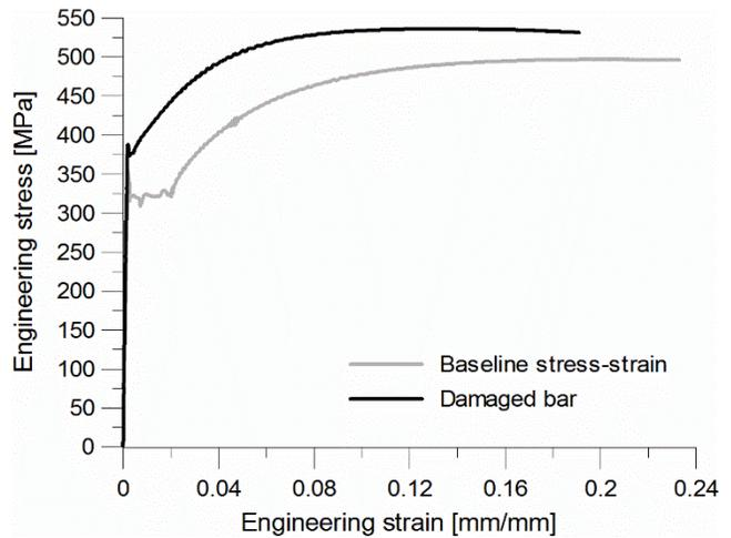
Fig. 14 Stress strain curve of the D2 damaged bar and a virgin bar of same grade and diameter.
