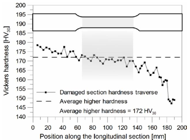
Fig. 8 - Vickers hardness traverse profile of the D2 damaged bar.
