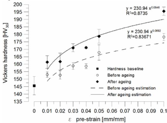
Fig. 11 Hardness versus pre-strain calibration curve for diameter 25 mm grade 300.
