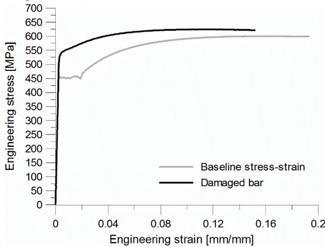
Fig. 13 Stress strain curve of the D1 damaged bar and a virgin bar of same grade and diameter.
