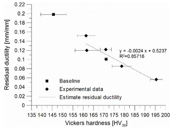
Fig. 12 Residual strain capacity versus Vickers hardness calibration curve for diameter 25 mm grade 300.
