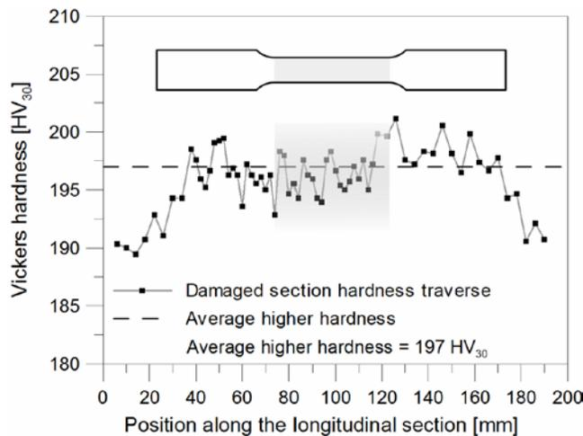
Fig. 7 - Vickers hardness traverse profile of the D1 damaged bar.
