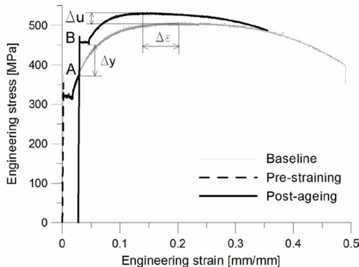
Fig. 2 Stress – strain curves of seismic Grade 300 reinforcing steel, as-received (un-aged), and pre-strained to 0.03mm/mm, aged for 4 hours at 100°C to simulate one year at 15°C and then re-loaded to investigate strain age effects.
