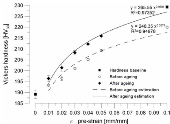
Fig. 9 Hardness versus pre-strain calibration curve for diameter 16 mm grade 430.
