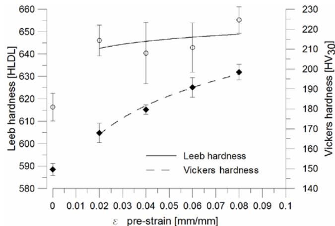
Fig. 3 Comparison Leeb and Vickers hardness versus pre-strain curves for NZ Grade 300E steel reinforcing bar.
