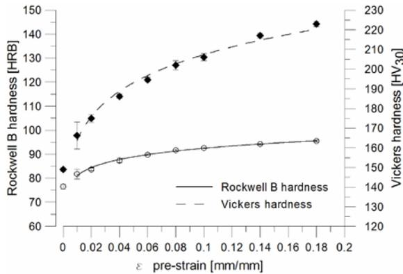
Fig. 4 Rockwell B and Vickers hardness versus pre-strain calibration curves for Grade 300E steel reinforcing bar.
