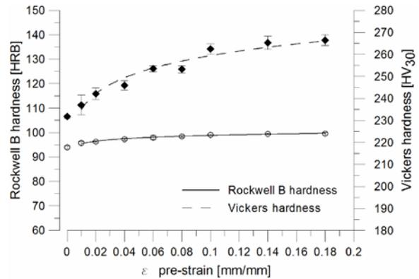
Fig. 5 Rockwell B and Vickers hardness versus pre-strain calibration curves for Grade 500E steel reinforcing bar.
