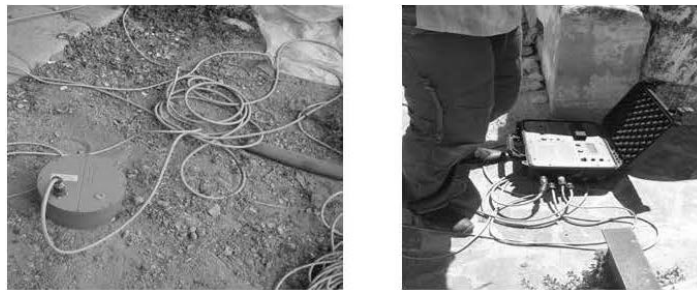
Fig. 2: Station CityShark II (right) and 3 components Lennartz 5 sec. Velocimeter (left)
