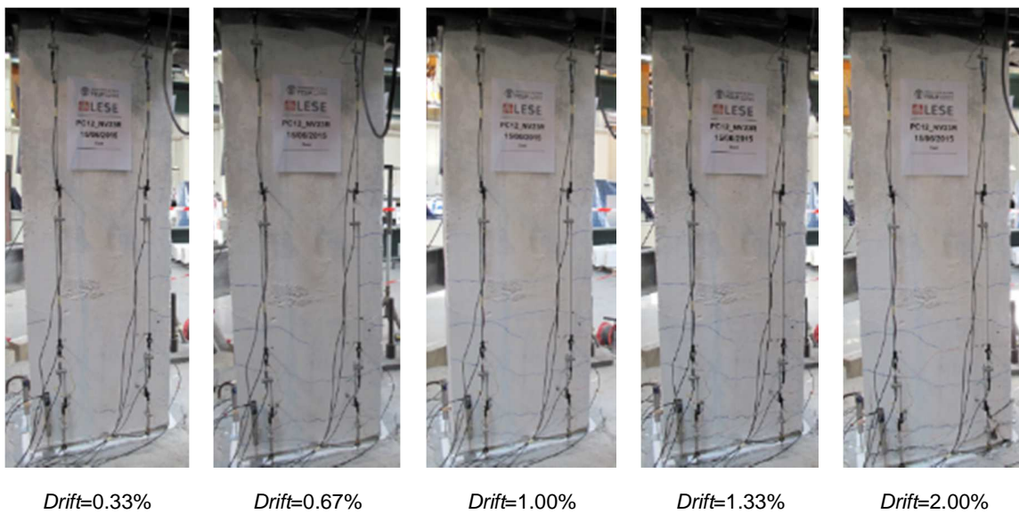
Fig. 7 – Damage evolution: PC12NV1B.
