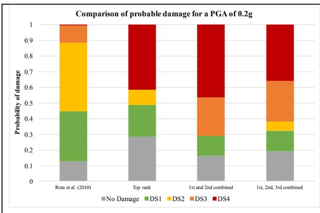
Figure 16 – Comparing probable damage of the URM class from the selected functions for a PGA of 0.2g
