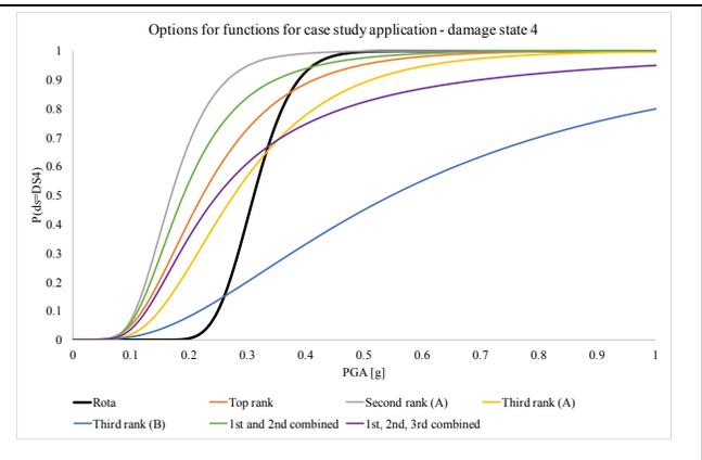
Figure 15 – Comparing existing function options – fourth damage state
