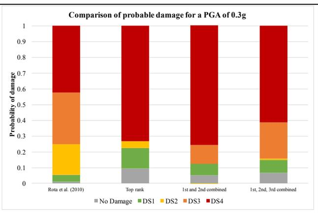
Figure 17 – Comparing probable damage of URM class from selected functions for PGA of 0.3g
