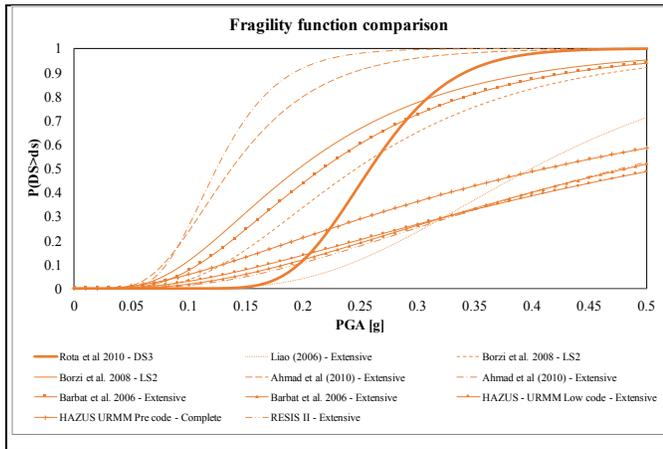
Figure 3 – Comparing results for an unreinforced masonry building class by Rota et al. [10] – third damage state
