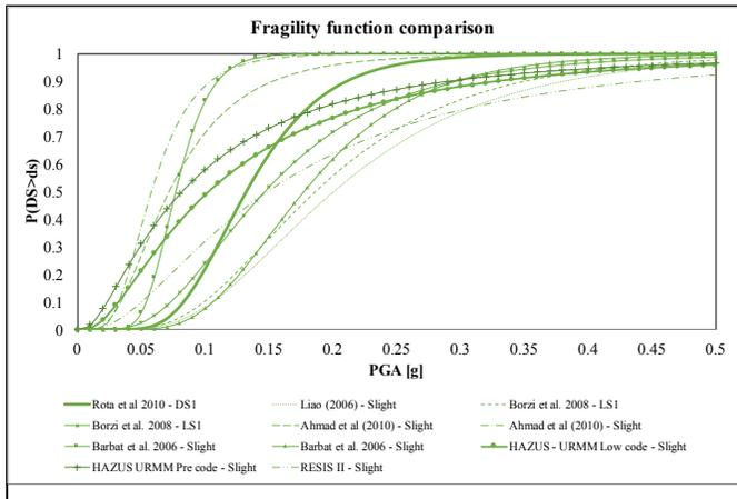
Figure 1 – Comparing results for an unreinforced masonry building class by Rota et al. [10] – first damage state
