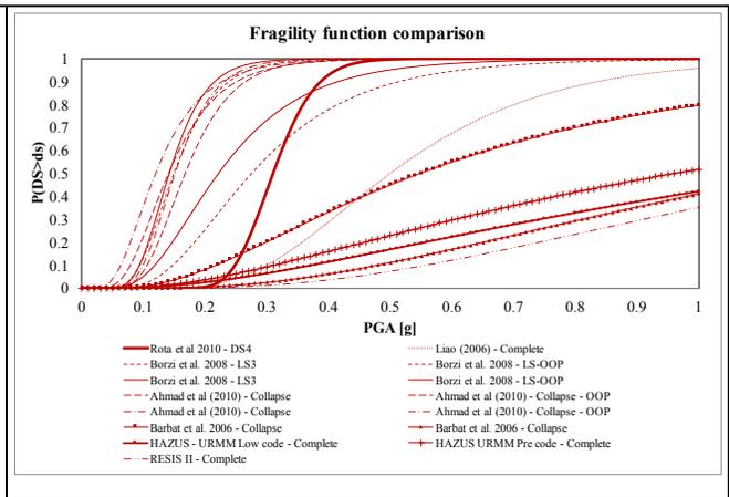
Figure 4 – Comparing results for an unreinforced masonry building class by Rota et al. [10] – fourth damage state
