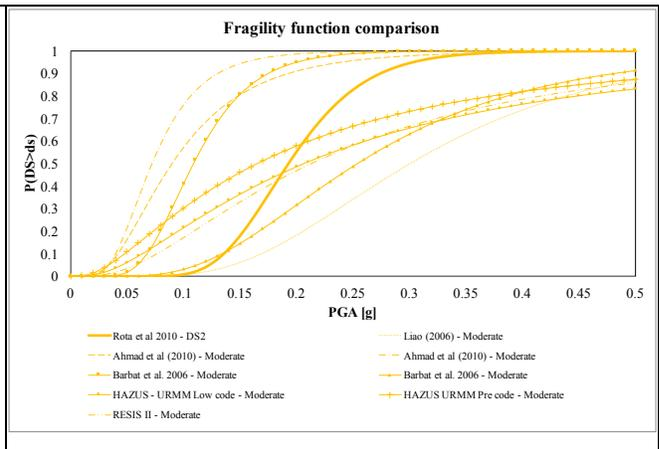
Figure 2 – Comparing results for an unreinforced masonry building class by Rota et al. [10] – second damage state
