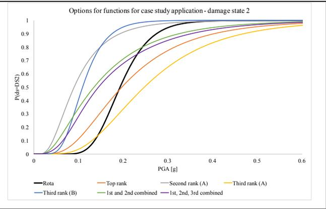
Figure 13 – Comparing existing function options – second damage state
