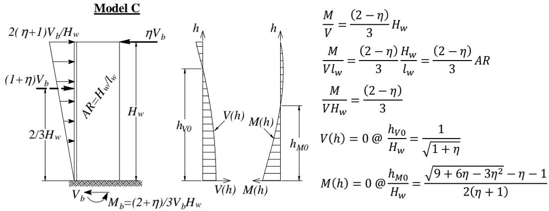
Fig. 10 – Response parameters of cantilever wall models under seismic loading.
