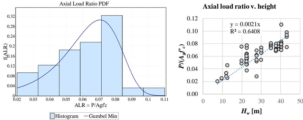
Fig. 8 – Axial load ratio distribution (ALR, left), and ALR correlation with building height.
