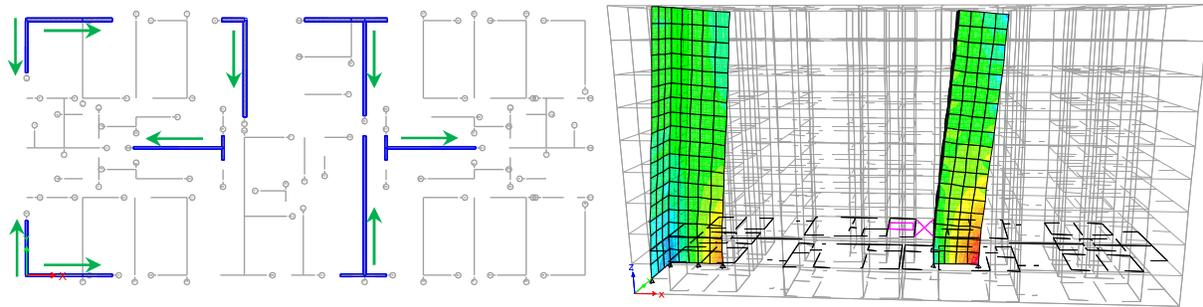
Fig. 4 – Isolation of flange-walls of interest in several direction for building 22 (left); vertical stress field on two flanged walls under lateral loading compressing the web (building 28).
