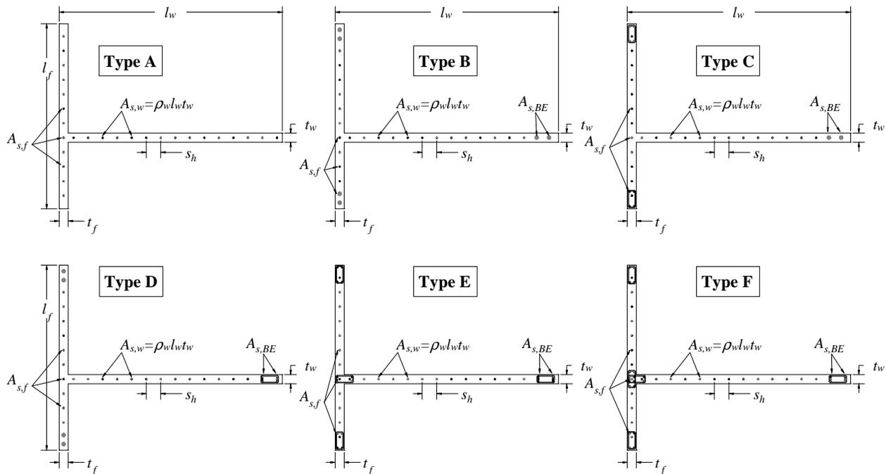
Fig. 7 –Types of reinforcement layout
