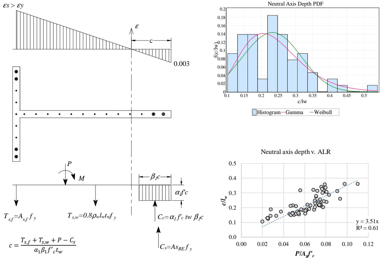
Fig. 9 – Compatibility and equilibrium in the cross section of flanged-walls under axial load and moment compressing the web end (left); normalized neutral axis depth distribution (top right); normalized neutral axis depth versus ALR (bottom right).
