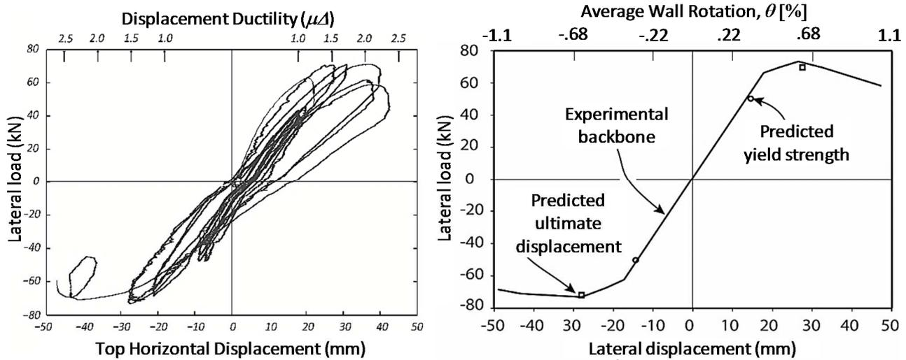
Fig. 14 – Hysteresis curve and corresponding envelope of response.
