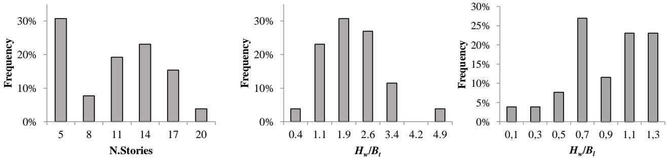
Fig. 2 – Global geometric variables: number of stories and building aspect ratio.
