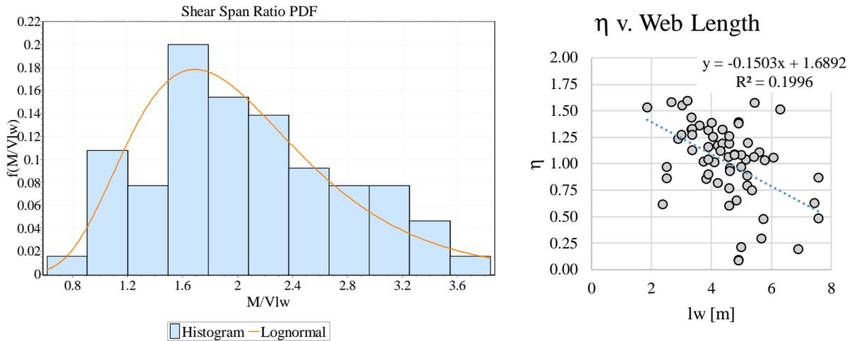
Fig. 11 – Shear span ratio distribution (left); coupling factor,  $\eta$ , versus web length relationship (right).
