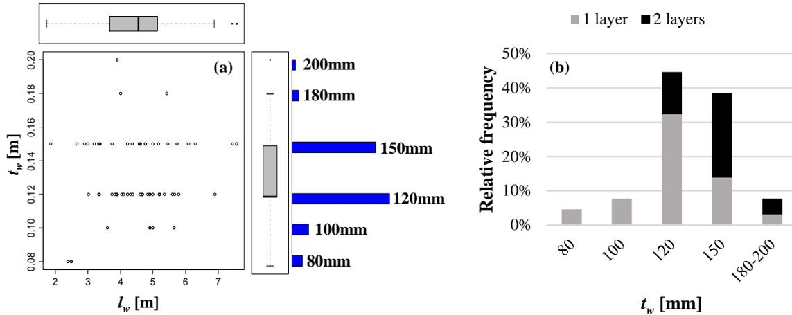
Fig. 6 – Web thickness and reinforcing layers: (a) thickness versus length of the wall; (b) number of web steel layers per wall thickness.
