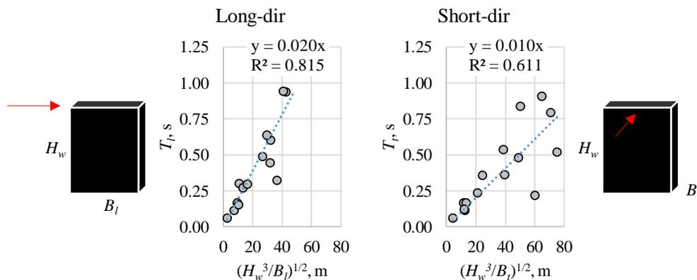
Fig. 5 – Fundamental period versus global geometric variables.
