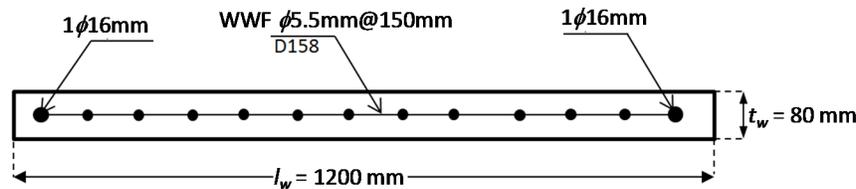
Fig. 13 – Detail of the wall specimen.
