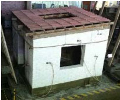
Fig. 2 - Adobe model on the shaking table, prior to testing
