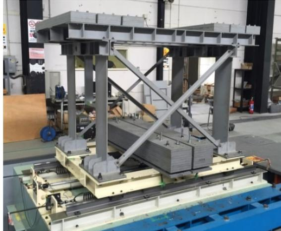
Fig. 4 – Base-isolated specimen with braces locked.
