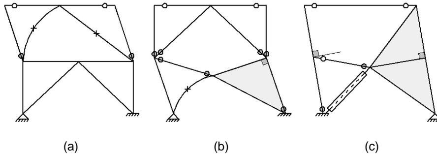
Fig. 4 – Schematic of plastic mechanisms of the test specimens:
