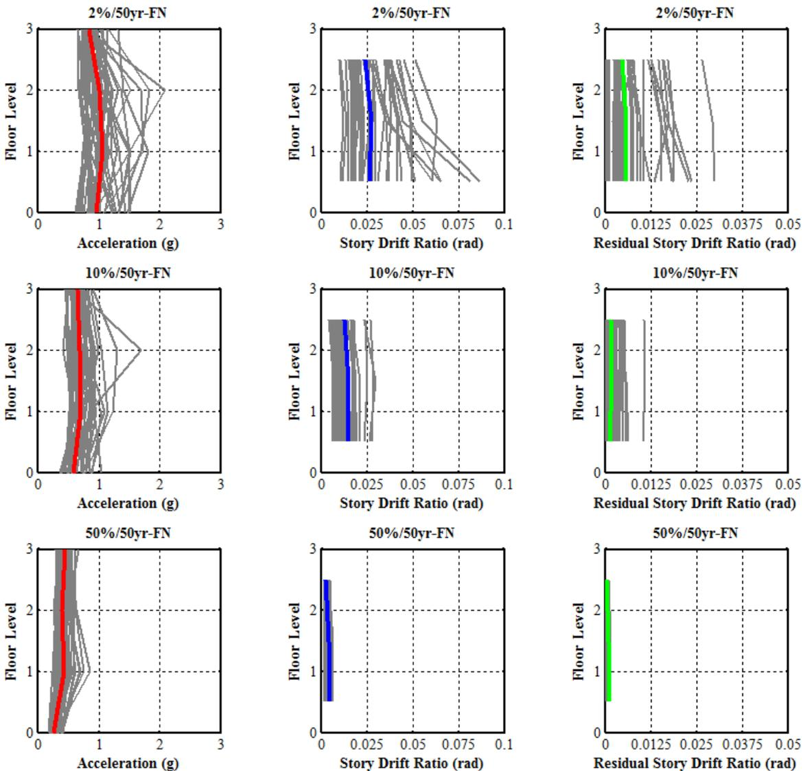
Fig. 9 – Engineering demand parameters and the median response: peak absolute acceleration, story drift ratio, and residual story drift ratio.
