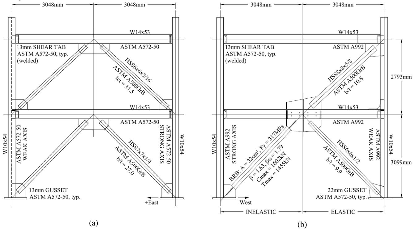
Fig. 3 – Test specimen schematic with dimensions, materials, and member sizes:
