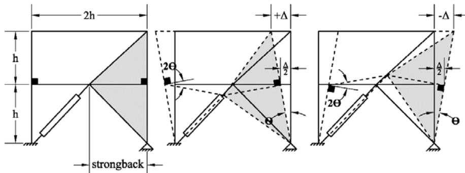
Fig. 5 – Idealized kinematic relations of strongback test with a lambda configuration (NCBF-B-3SB).
