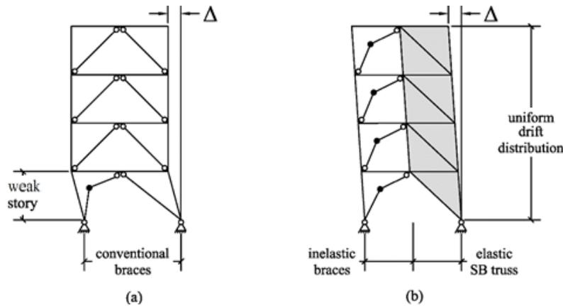
Fig. 1 – Examples of plastic mechanism: (a) conventional braced frame; (b) SB system.
