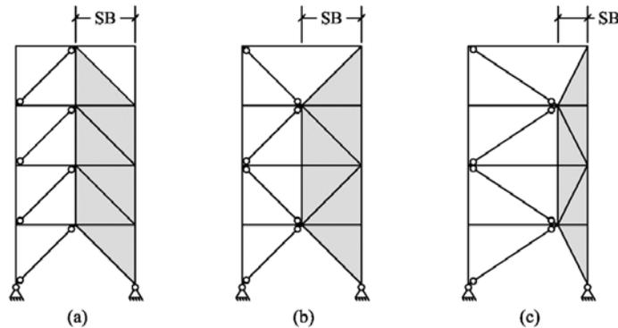
Fig. 2 – Possible SB configurations: (a) “chevron” SB; (b) double story X SB; (c) offset double story X SB
