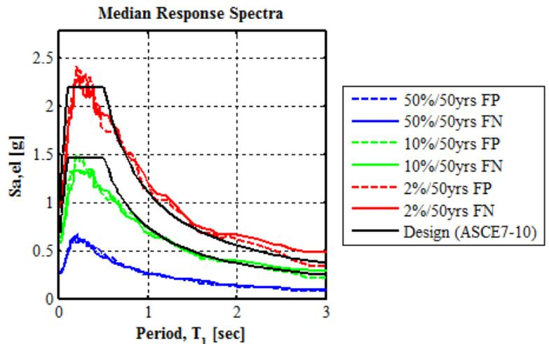
Fig. 8 – Median pseudo-acceleration of records and code-stipulated design spectra.
