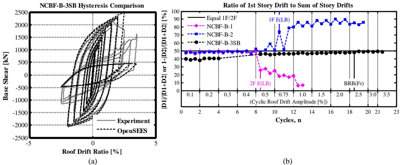
Fig. 6 – (a) NCBF-B-3SB comparison of numerical and experimental results of global hysteresis; (b) Comparison of the weak story tendency at peak cyclic amplitudes (Fr = fracture; LB = local buckling).
