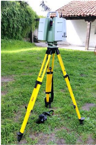
Fig. 13 (left) – USF’s Leica ScanStation C10 laser scanner, photo by author Fig. 14 (right) – “Scan plan” record of scanning locations throughout site.
