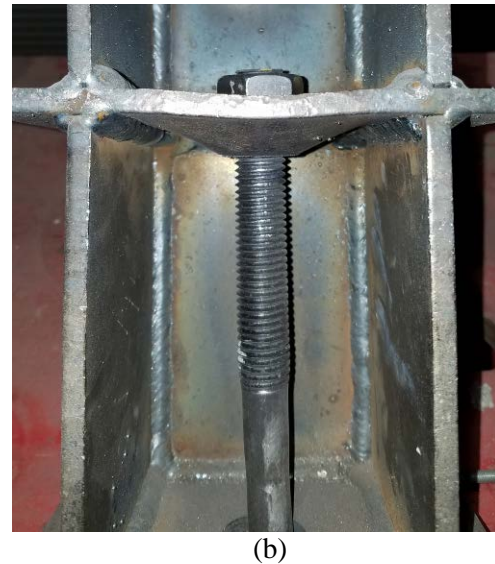
Fig. 6 – Single Anchor Tests: (a) Single Anchor Failure Displacements; (b) Top Plate Bending [Yielding Chair]
