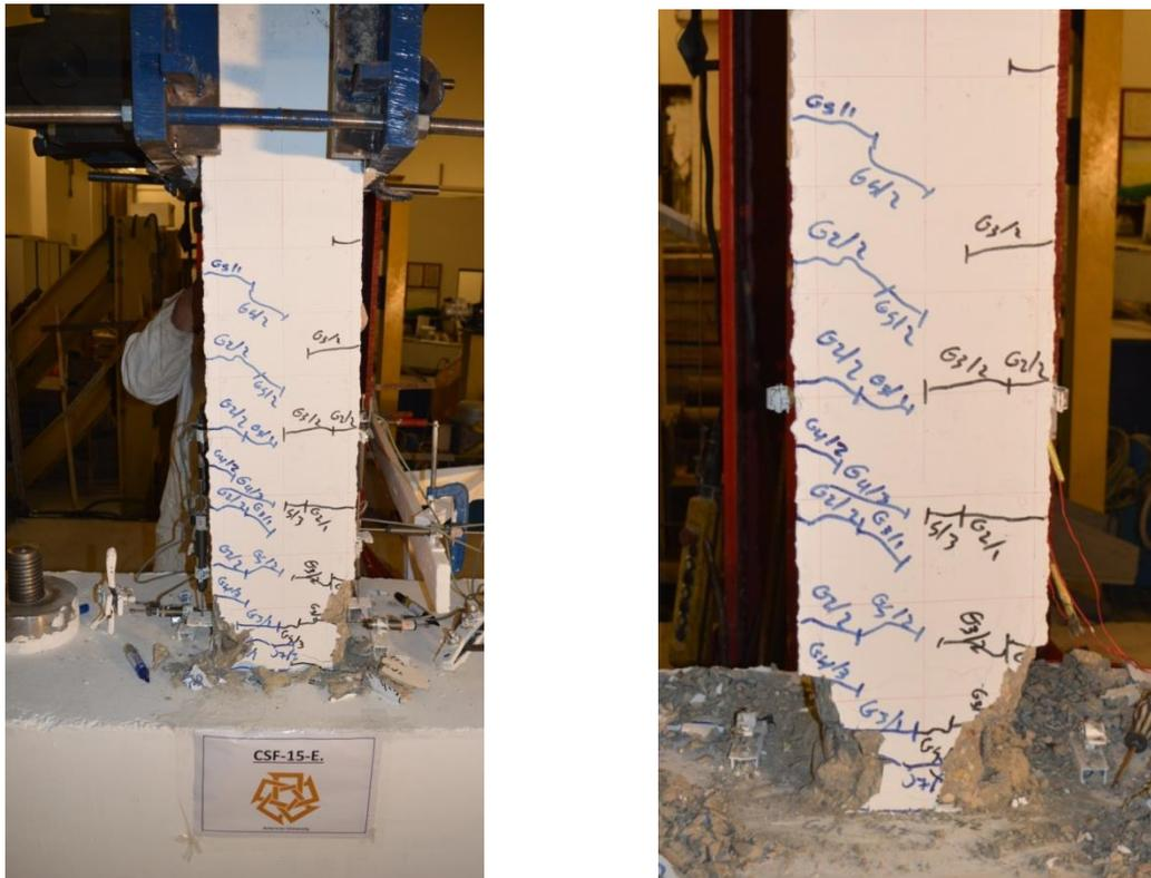
Figure 5: Failure mode of specimen F15
