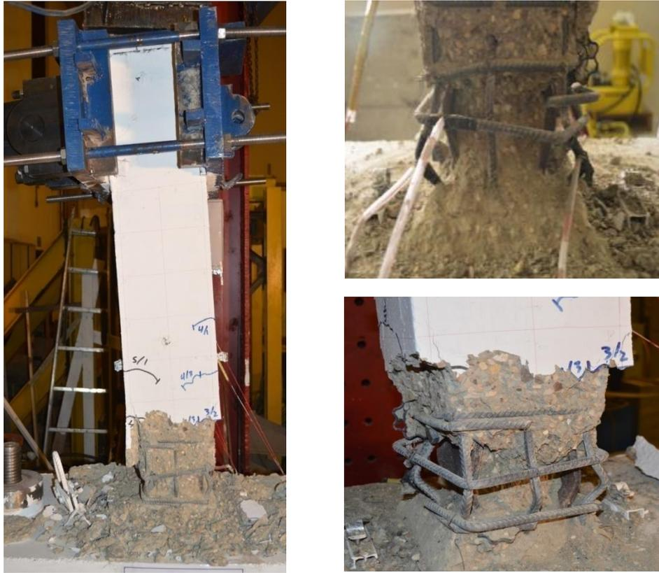
**Figure 7:** Failure mode of specimen F80
