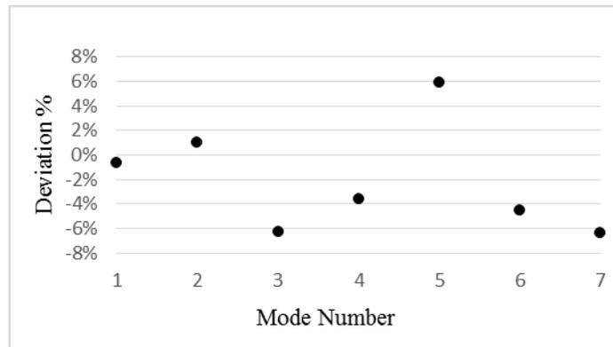
Fig. 14 - Identified vs. calculated eigenfrequencies deviations with updated model parameters.
