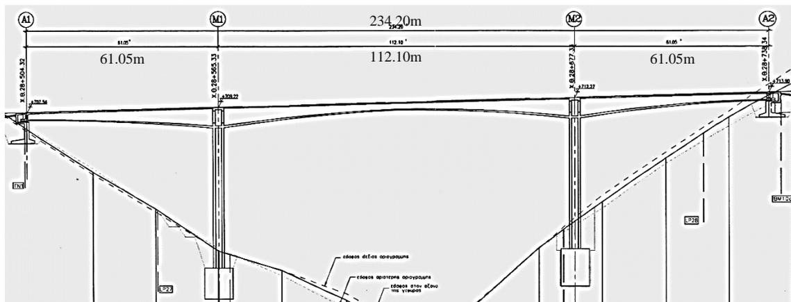
Fig. 2 – Vertical section of the bridge, on deck axis.
