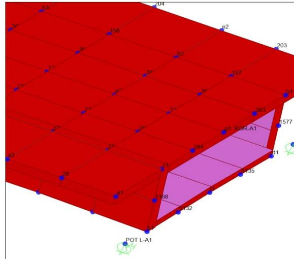
Fig. 11 – Substitution of end cap with body constraint including end nodes and pot-bearings nodes.
