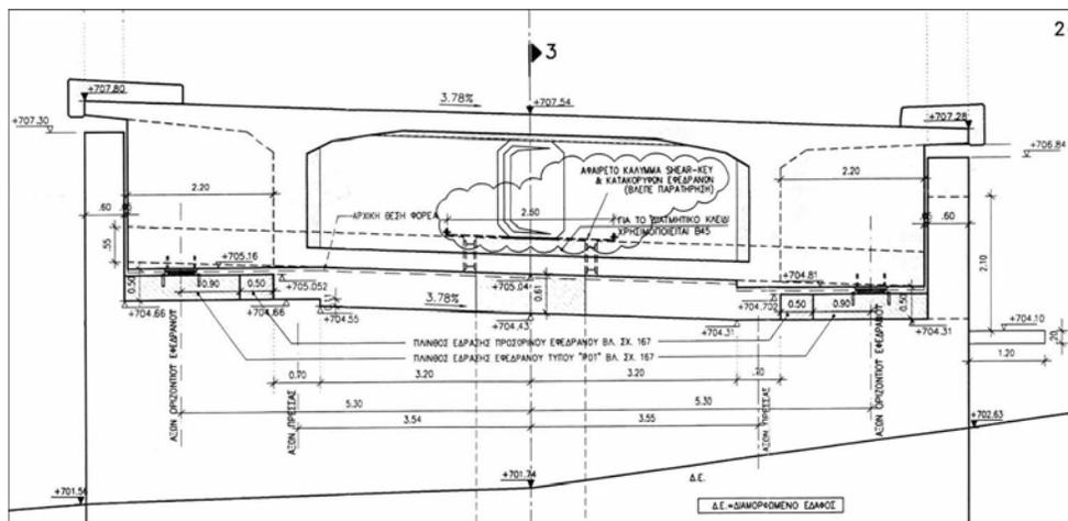
Fig. 5 – Section at the abutments illustrating the pot bearings the shear key and the end cap.
