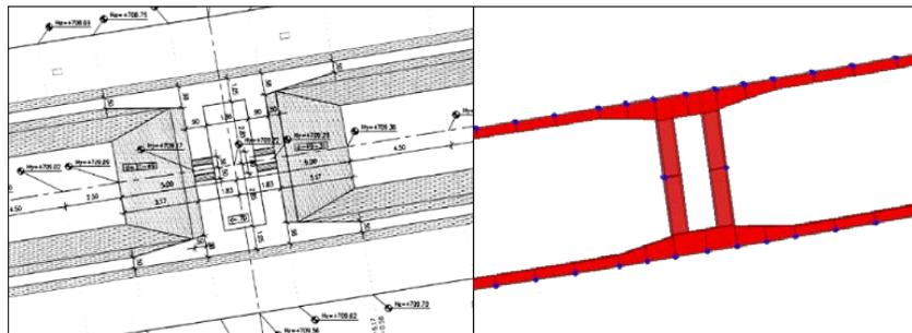
Fig. 8 – Horizontal section at the pier to deck connection (left) and corresponding FE connectivity (right).
