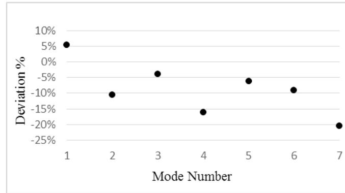
Fig. 13 – Identified vs. calculated eigenfrequencies deviations with initial model parameters.
