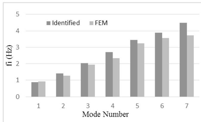
Fig. 12 – Identified vs. calculated eigenfrequencies values with initial model parameters.
