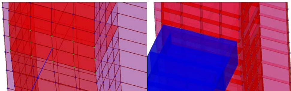
Fig. 10 – Beam FE (blue) connection of pier to shells Fes (red) of the deck. In green the nodes of the body constraint.
