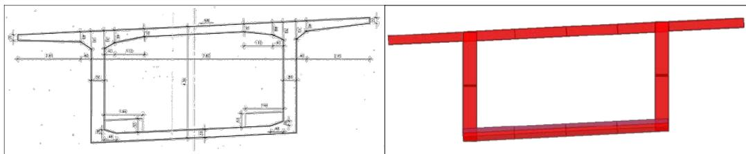
Fig. 9 – Typical deck's box section and corresponding FE model simulation.
