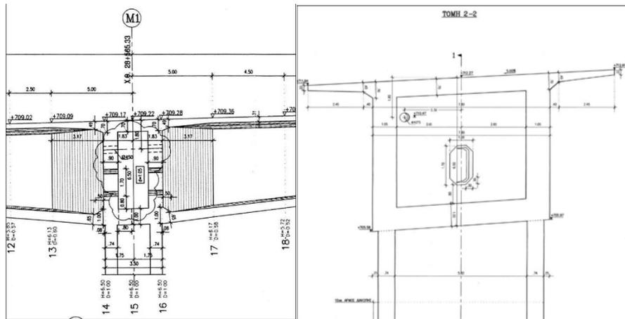
Fig. 6 –Longitudinal (left) and transverse (right) sections at the pier to deck connection.
