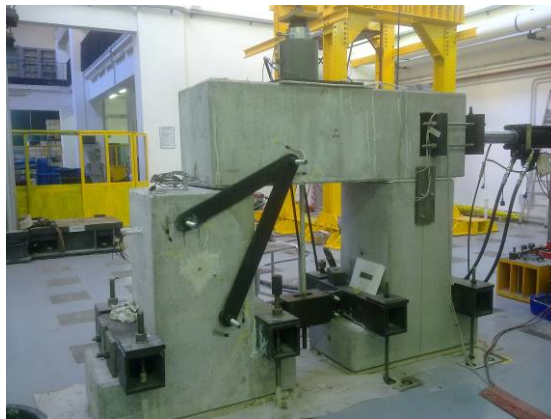
Fig. 3 - Retrofitting system configuration: test setup
