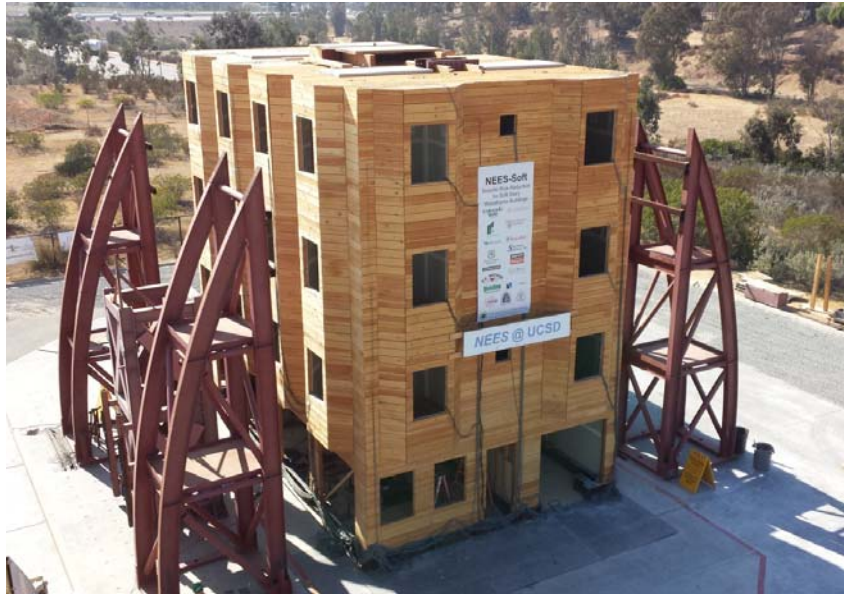
Figure 5 Full-scale four-story wood-framed test specimen on shaking table at NEES-UCSD.
