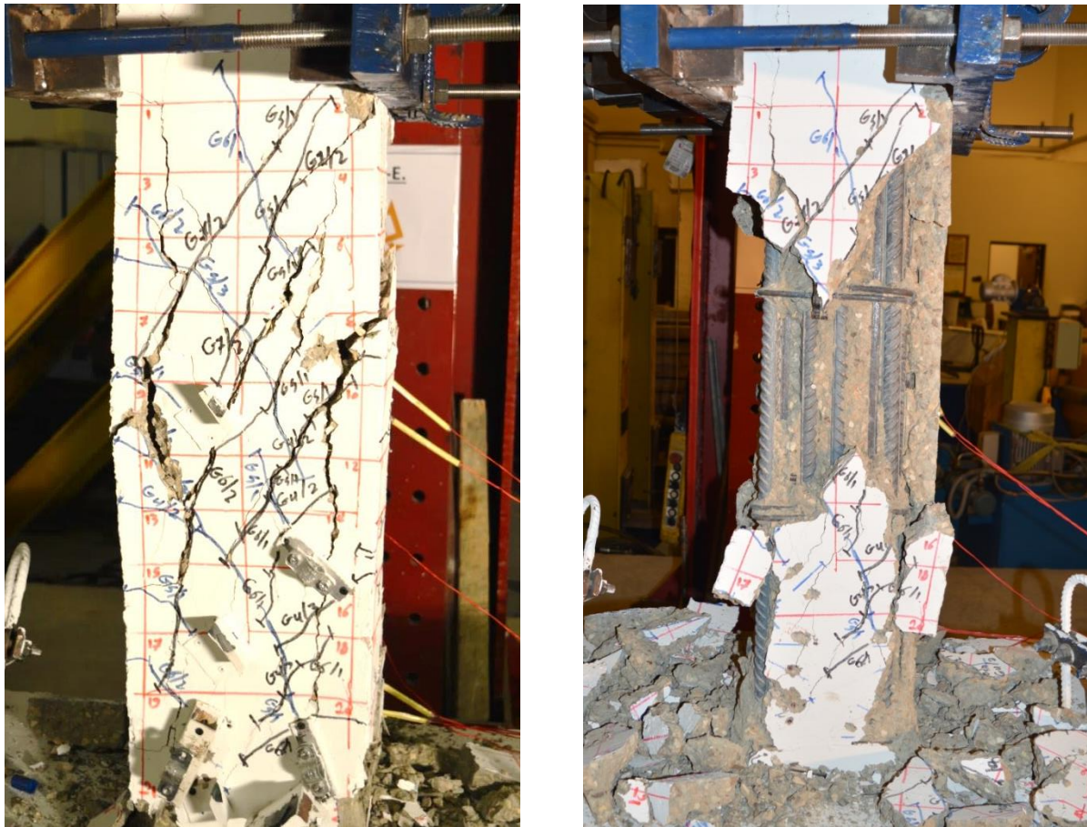
Figure 5: Failure mode of specimen S40
