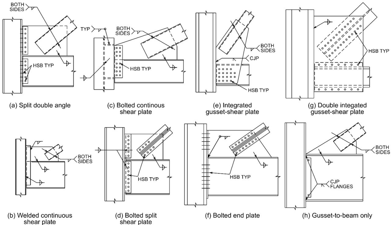
Fig. 2 – NCBF connection configurations
