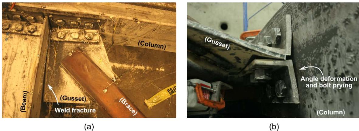
Fig. 6 – Specimen 2 (a) gusset-plate connection at 3.1% drift range and (b) angle deformation at 6.2% drift range
