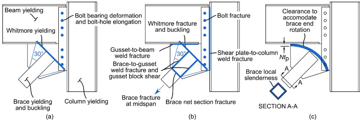
Fig. 1 – Concentrically braced frame (a) yielding mechanisms, (b) failure modes, and (c) geometric limits
