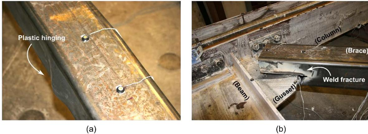
Fig. 5 – Specimen 1 (a) brace midspan and (b) brace end at 1.3% drift range
