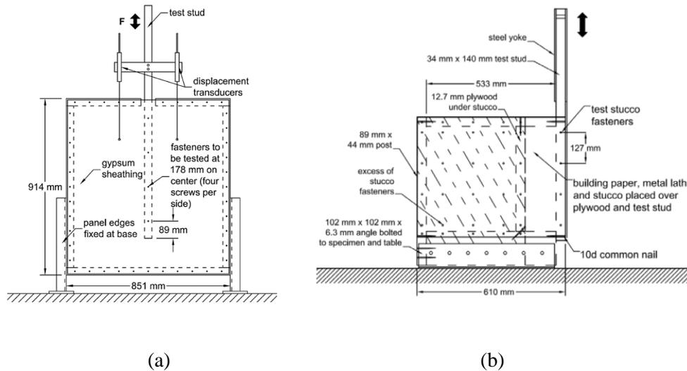
Fig. 3 –Test Setup: (a) Gypsum Connector Tests [7] and (b) Stucco Connector Tests [10]
