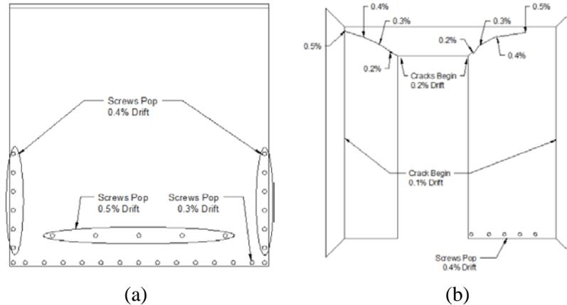
Fig. 5 –Damage Progression Unibody Walls: (a) GYP – GYP, (b) GYP – GYP (wall returns, door opening) [11]
