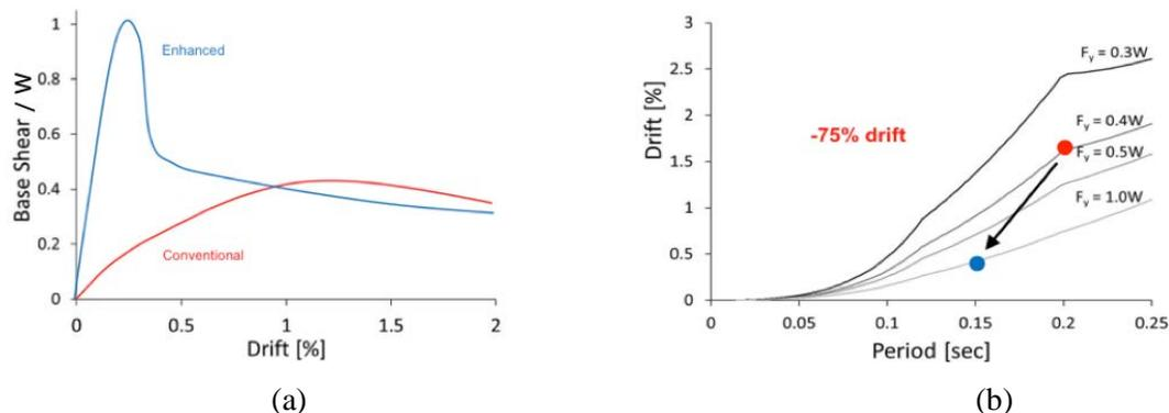
Fig. 1 – Unibody vs. Conventional: (a) Normalized base shear versus drift response and (b) drift [6]
