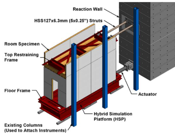
Fig. 6 – Unibody room test setup [13]
