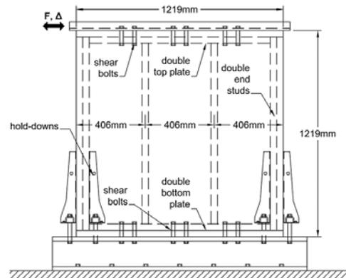
Fig. 4 – Test Setup for Small Walls [7]
