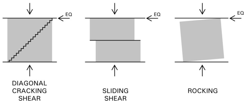
Fig. 7 - Masonry wall failure modes
