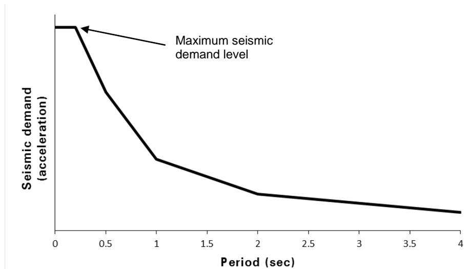
Fig. 4 - Example seismic demand response spectrum
