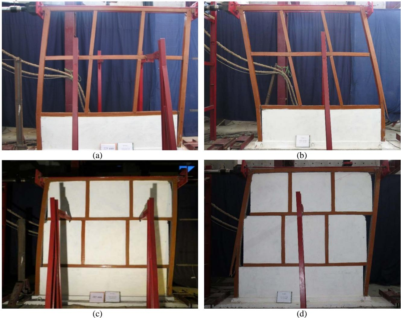
Fig. 6 – Assam-type housing frame wall tested specimens: (a) Frame 1 during cyclic loading, (b) Frame 1 at the end of monotonic loading, (c) Frame 2 during cyclic loading, and (d) Frame 2 at the end of monotonic loading
