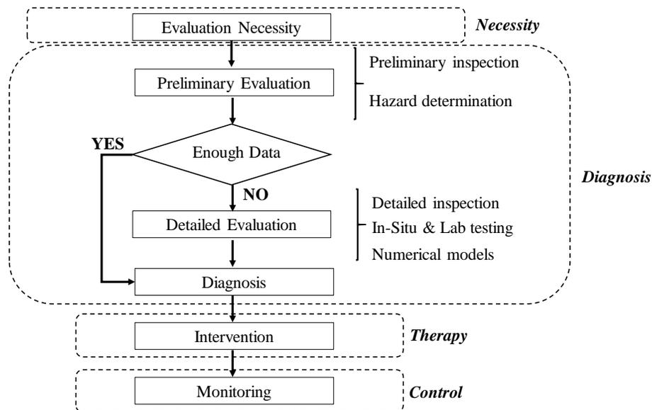
Fig. 1– Schematic view of a structural intervention in heritage buildings (adapted from [1])
