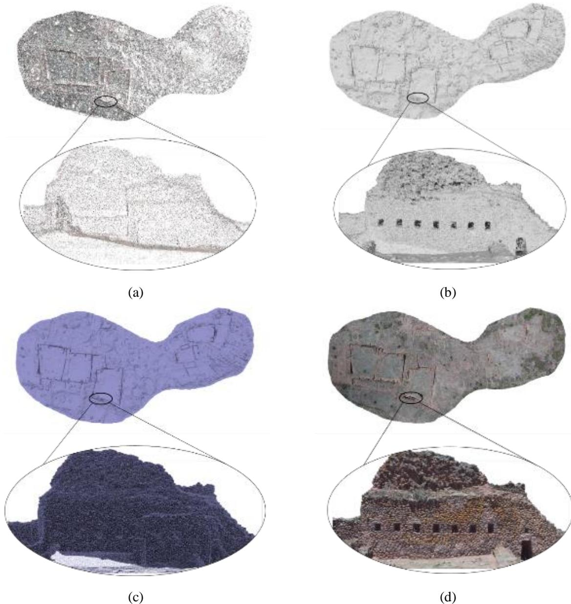
Fig. 3–Process of 3D model generation: a) image alignment and spread point cloud generation; b) generation of dense cloud; c) generation of triangular mesh; and d) generation of the texturized model
