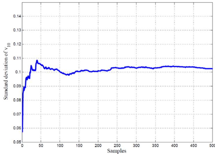
Fig. 4 – Convergence of the standard deviation of top floor velocity ( $\sigma_{\dot{x}}$ ).
