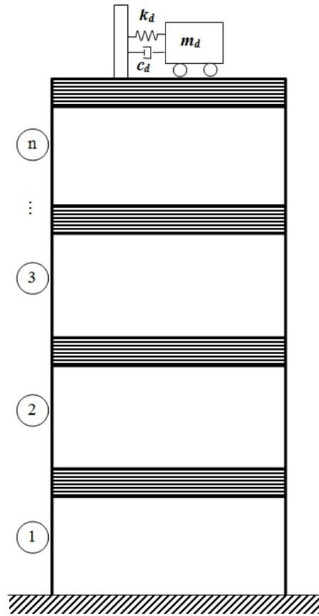
Fig. 1 – n-DOF building with single TMD on the top floor.
