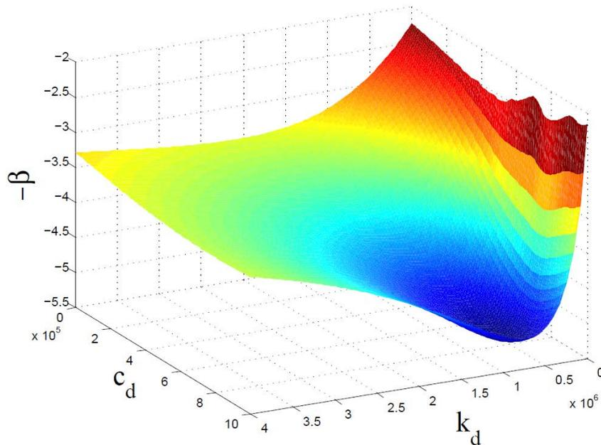
Fig. 5 – Objective function in the design space for the robust optimal design of a TMD (case (iii)).
