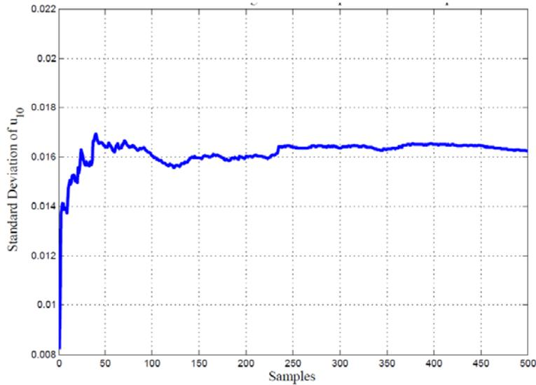
Fig. 3 – Convergence of the standard deviation of top floor displacement ( $\sigma_x$ ).
