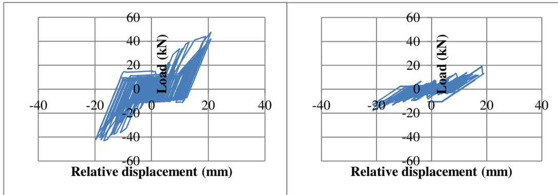
Fig. 7 – Response hysteresis of the model with optimized resistance in height,  $\alpha=0.2$ . First floor at left and fourth floor at right.
