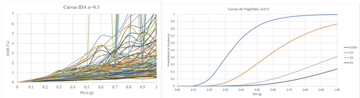
Fig. 10 – (a) Drift vs. PGA for  $\alpha=0.5$
