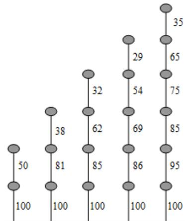
Fig. 1 – Proposed distribution (%) of floor resistance, for buildings from two to six floors in height.
