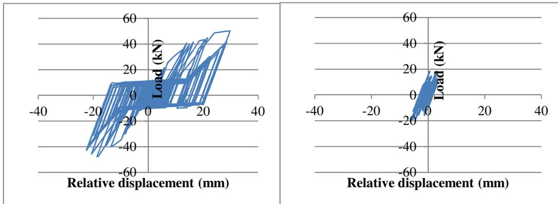
Fig. 6 – Response hysteresis of the model with uniform resistance in height,  $\alpha=0.2$ . First floor at left and fourth floor at right.
