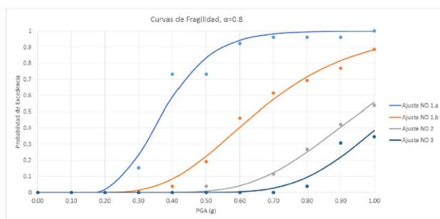
Fig. 2 – Fragility Curves for  $M_w \geq 7.5$
