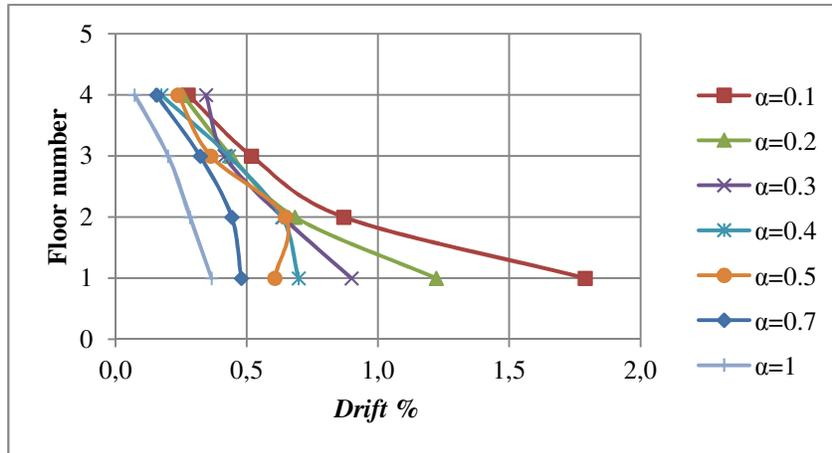
Fig. 4 – Distribution of maximum drift for a building with uniform shear capacity in height.
