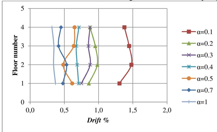
Fig. 5 – Distribution of maximum drift for a building with optimized shear capacity in height.
