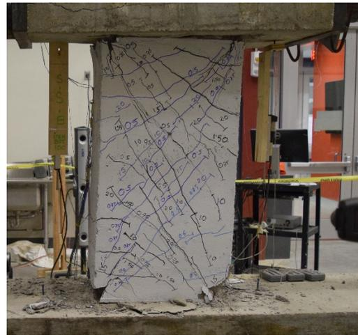
Fig. 7 – Deformation of CB2 at a chord rotation of +5.2%
