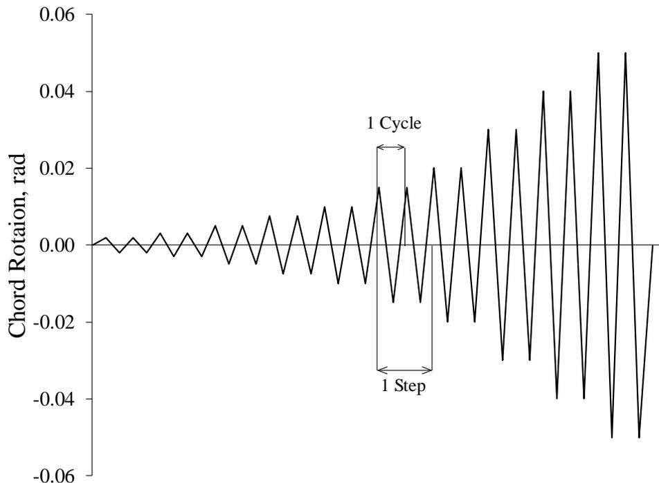
Fig. 5 – Target loading protocol
