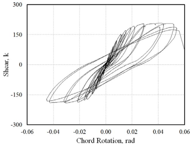
Fig. 6 – Shear versus chord rotation for CB2
