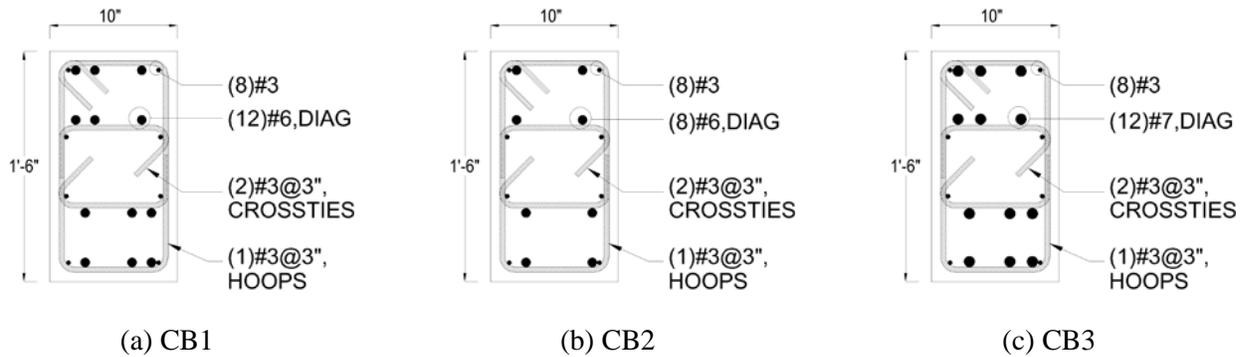
Fig. 2 – Coupling beam cross-sections near wall intersection
