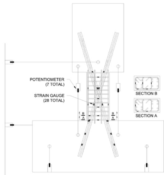
Fig. 4 – Instrumentation
