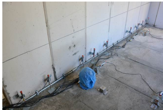
Fig. 9 – Measurement of the wall panel rocking
