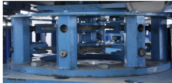
Fig. 3b1. Tested innovative energy dissipation devices (HC-EDD) of horizontal HC-type
