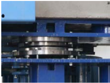
Fig. 3a1. Tested (DSRSI) double spherical rolling seismic isolator
