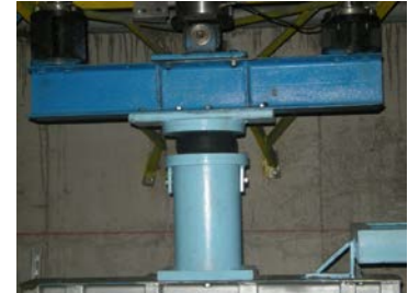
Fig. 3c1. Tested displacement limitation devices (R-DLD)
