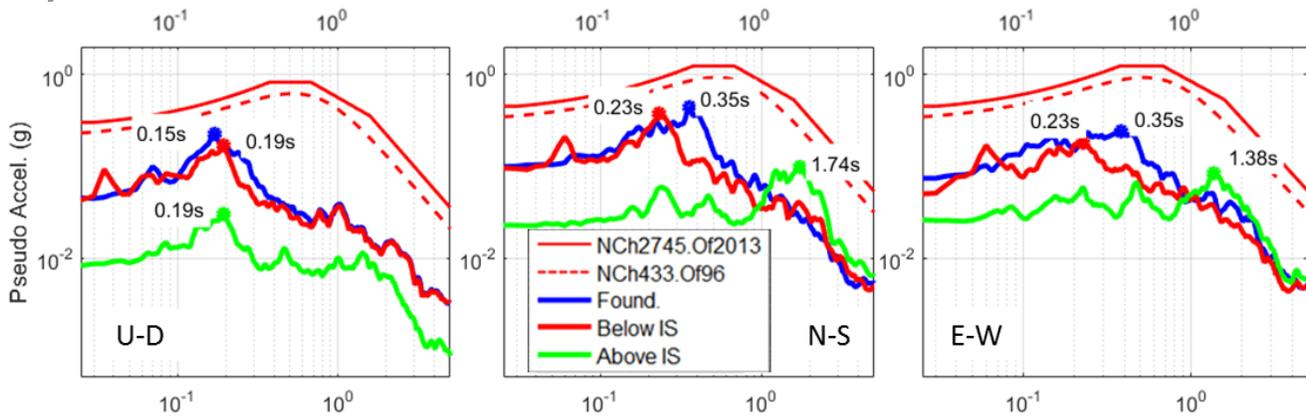
Fig. 6 - Elastic Spectra obtained using the measured accelerations in the El Carmen Hospital, the NCh433 D61 spectrum and the NCh2756 Spectrum. (IS: Isolation System)
