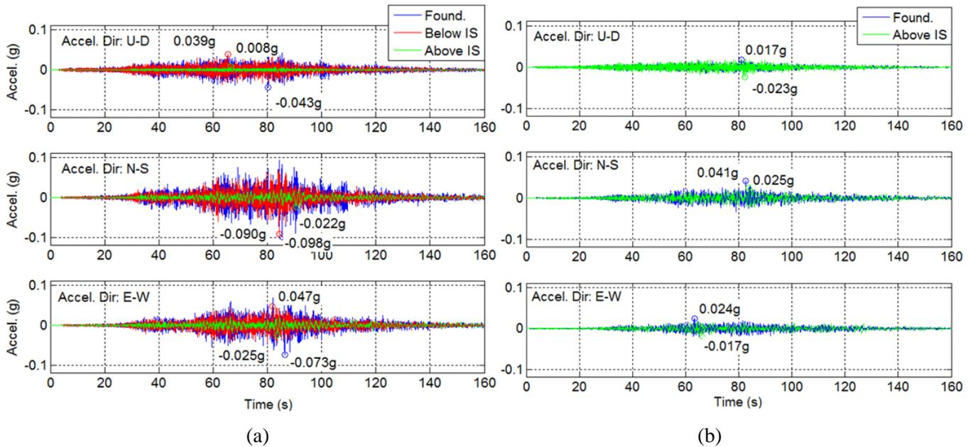
Fig. 5 – Measured accelerations for all sensors and all directions (a) ECH project (b) LFH project.
