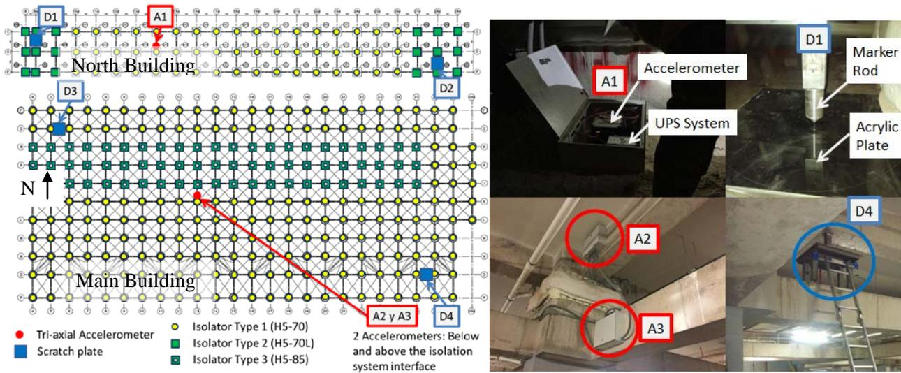
Fig. 1 – Location of the measurement devices for the ECH.
