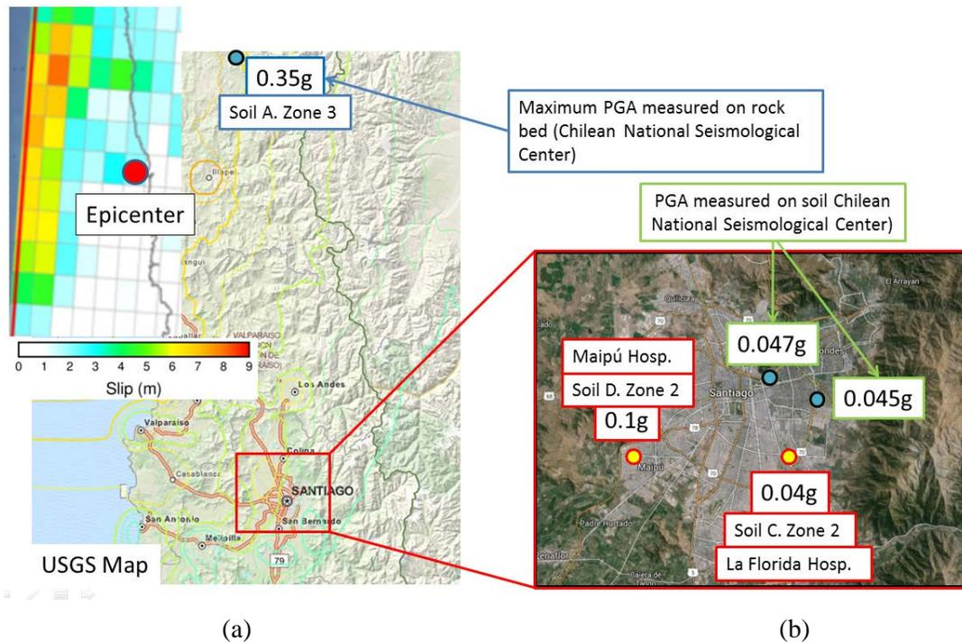
Fig. 3 – Fault slip profile and PGA levels for the Sep 16, 2015 Mw 8.3 earthquake [9]. (a) PGA near the epicenter (b) PGA levels at different locations in Santiago (Chile).
