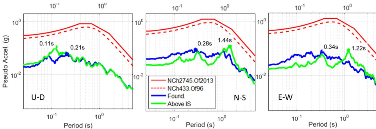
Fig. 7 - Elastic Spectra obtained using the measured accelerations in the La Florida, the NCh433 D61 spectrum and the NCh2756 Spectrum. (IS: Isolation System)
