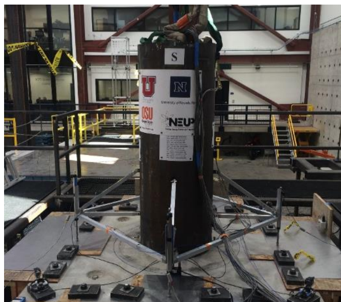
Fig. 2 – Final test setup of MPC specimen on shake table
