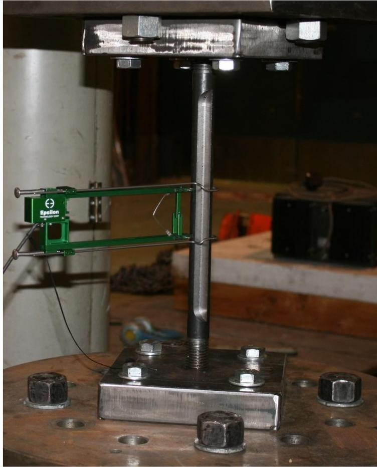
Figure 4: Tensile test setup of groove type dissipaters
