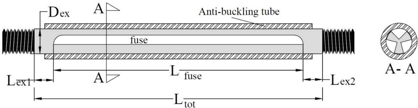
Figure 1: Schematic figure of a groove type dissipater
