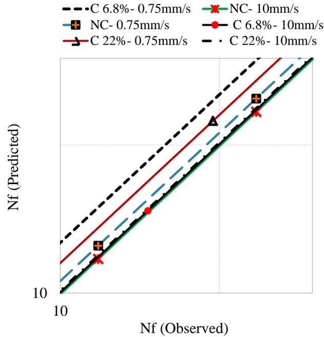
Figure 6: Comparison low cycle uniaxial fatigue life of the dissipaters with varying degree of corrosion predicted by 4-PC, and experiment (observed) with deformation rate of 10 mm/s and 0.75 mm/s
