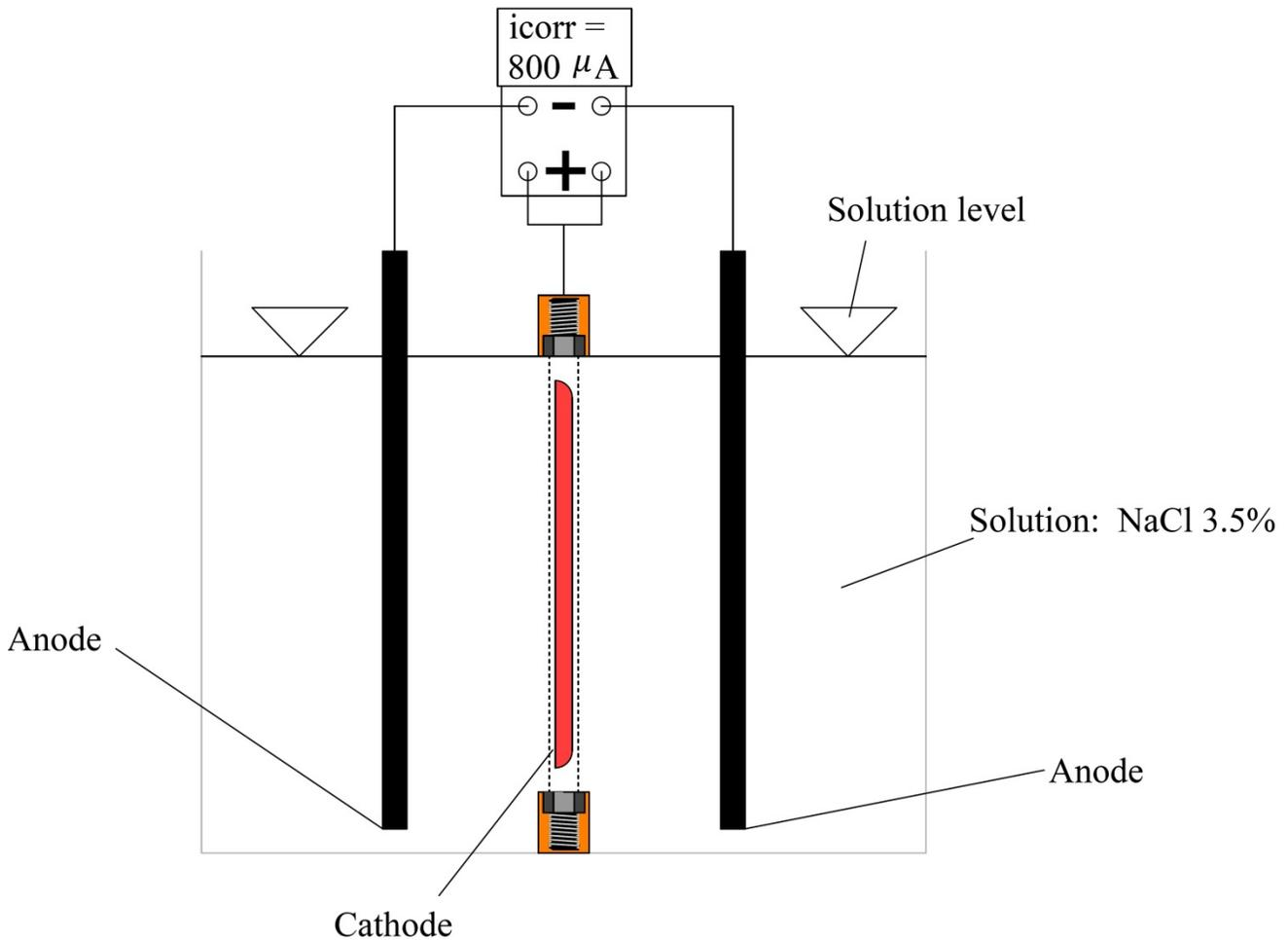
Figure 3: Details of corrosion test setup of the dissipaters
