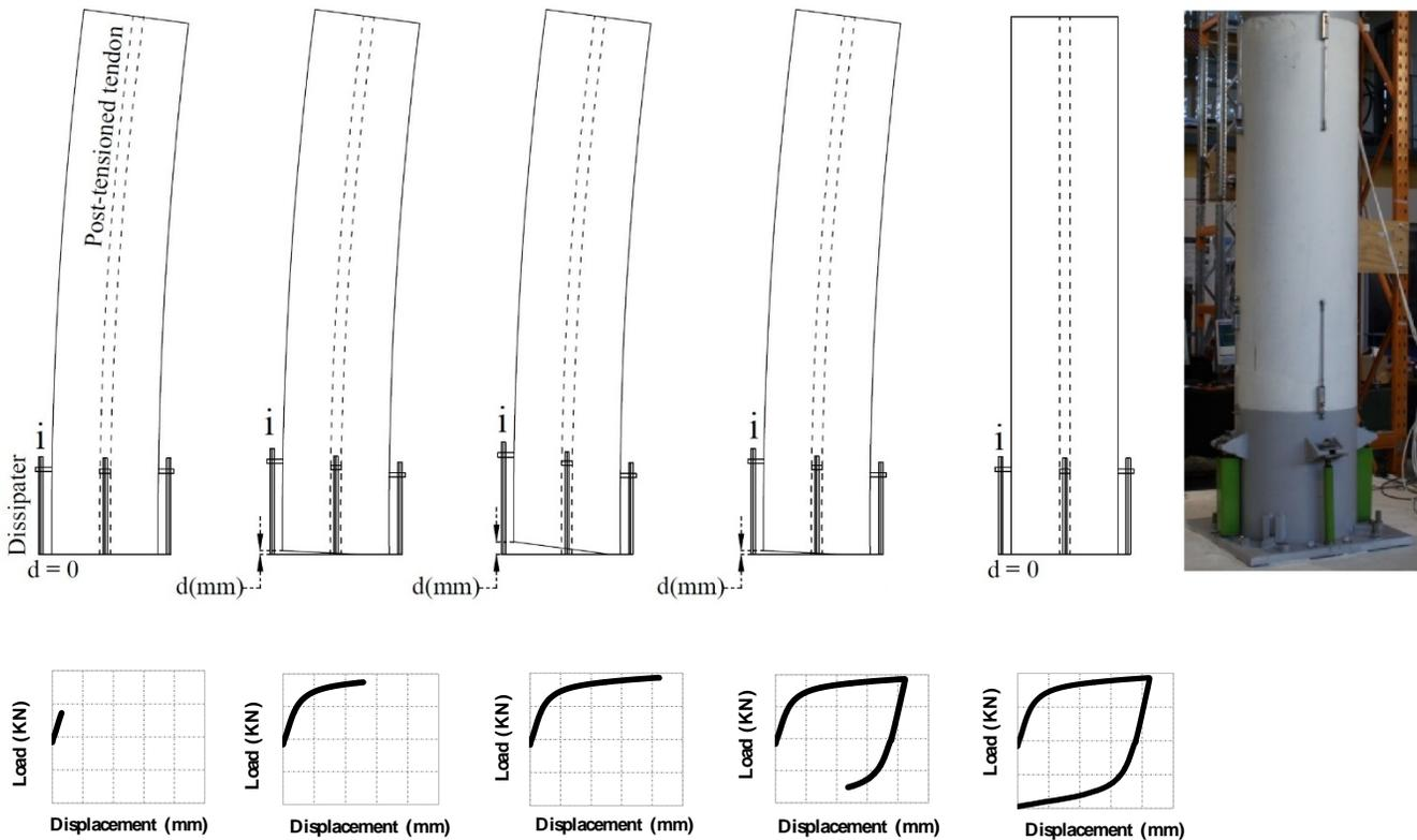
Figure 2: Schematic rocking bridge pier, stress-strain of dissipater i with a photo of a rocking bridge pier
